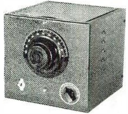
Rear and panel views of the QRM dodger. Each part has been so placed to minimize the chance of inter-element reaction. The air condenser has been used to add stability.
