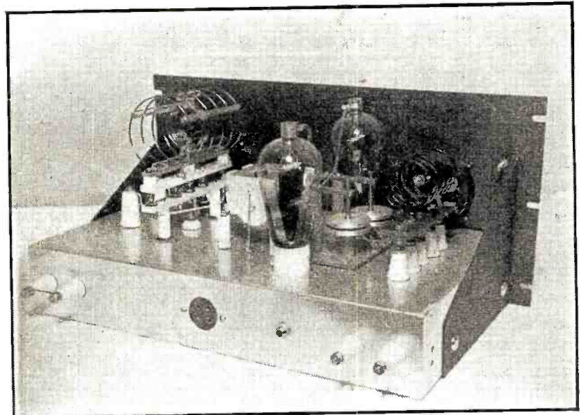
FRONT AND REAR VIEWS OF THE 112-WATT R.F. FINAL STAGE
