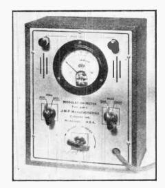
mits the amateur to check his positive and negative peaks, hum level and carrier shift. This is the type AM-1 modulation meter put out by the JMP Manufacturing Company and is shown in the accompanying photograph. (Turn to page 379)
