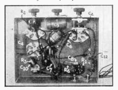
glow at a dull cherryred color in a dim light. Do not turn the rheostat above this point; the filaments of all 2-volt tubes are rather delicate and operation at too high temperatures will either burn them out or shorten their useful life. R1 is not shown in the photograph and may be omitted if a 2 volt shortage battery or an "Air Cell" battery is employed. A 1 ohm fixed resistor may then be substituted.
