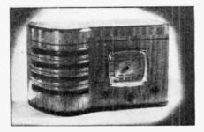
standard broadcast band and police and amateur ranges. Its rated power output is 3 watts. It has automatic volume control, and uses a 6½-inch dynamic type speaker.
