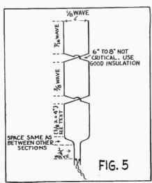
inch short of this length and clip the twisted pair feeders onto the matching section about four inches short of half the antenna length. The distance from the bottom of the antenna rod down to one clip, across to the other clip and up again to the open end of the matching section will be about the length of the antenna rod.
