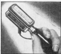
made, is available with either a high or low impedance type output transformer. It can be used as a hand or desk microphone or installed on a regular floor stand. As its name implies it is designed to be a handy microphone for many purposes. Its response is rated flat from 60 to 7500 cycles per second and an output 3 db below the standard size velocity transmitter.
