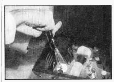
steel and is magnetized for picking up small objects. The composition handle holds two standard flash-light cells.
