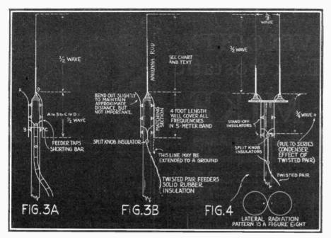
CONSTRUCTION DATA FOR USING THE "J" ANTENNAS
