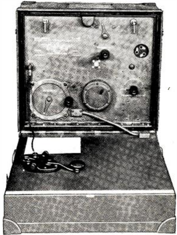
TRANSMITTING AND RECEIVING Close-up of the set, showing key and tuning controls
