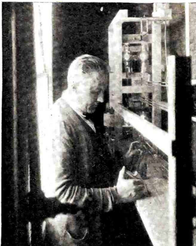
MEASURING THE SIXTY-EIGHT CENTIMETER WAVE Dr. Lindenblad measuring the sixty-eight centimeter wave with a small wavemeter. The length of the wire is equal to one-half of the wavelength
