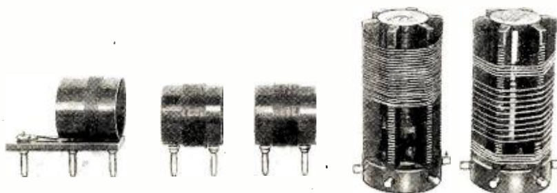
Figure 7. The coil winding data and, below, the coils. These are (left to right) the oscillator grid, oscillator plate, buffer plate, intermediate plate (and p.a. grid), and p.a. plate (and antenna) coils
