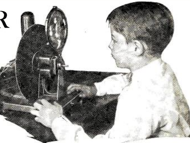
The radiovisor completed and in operation. The model shown here differs from the one described only in the use of a metal base instead of wood
