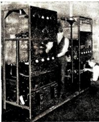
In the DeForest Radio Company's plant at Passaic, N. J., are to be seen the two units of the 1-kilowatt, crystal controlled short-wave transmitter to be used to contact the Nautilus
