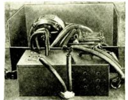
(Right) An interference suppresser attached to a sign flasher. At the right of the motor may be seen the make-and-break contacts, which are miniature "static" broadcasters
