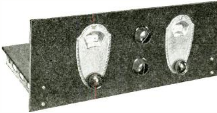
Two tuning controls, a volume control and a regenerator control make the operation of this set easy
