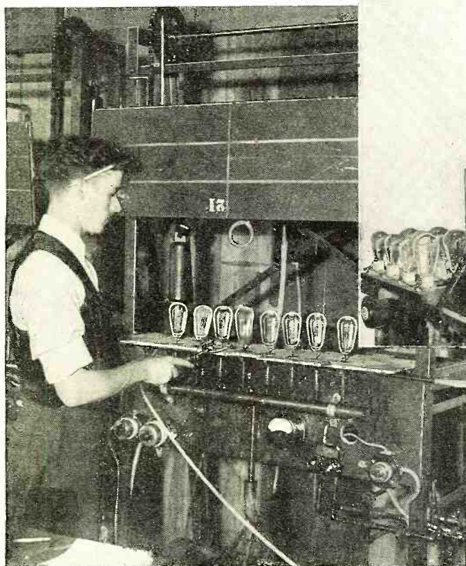
¶ Fig. 9—Another type of evacuating apparatus, with the furnace door raised to show the tubes in position
