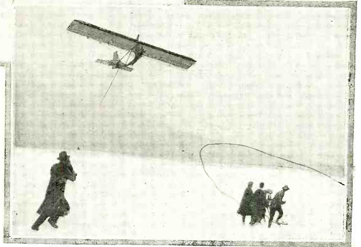
In the center we have the glider lifted into the air by the pull of the runners, the "shock-cord" slackening as the glider gains speed. In the final view the glider is free, with its tail rope in the air and the shock-cord falling to earth. The pilot is now "on his own."
