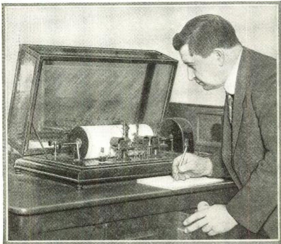
Dr. Scarr, whose frank comment on the folly of the "radio-weather" theory appears on the following page, is here observing the automatic machines which make a record in ink of every minute's weather at New York, year in and year out.
