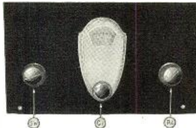
The short panel, with handsome illuminated vernier dial, and the two controls required by every regenerative circuit.
