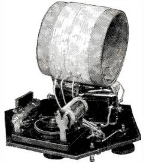
The layout of Mr. Thompson's crystal set (see first column) on its six-sided front panel.
