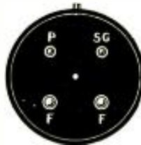
End view of the tube base, showing the arrangement of the contact pins. P, plate; FF, filament; SG, screen grid.
