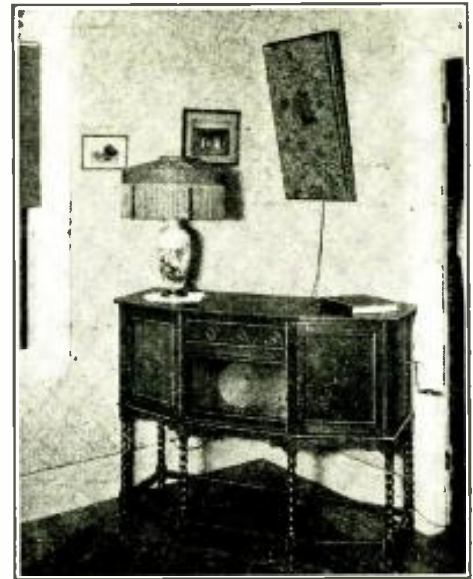
The electrified phonograph in its cabinet. The output may be connected to either the balsa-wood speaker on the wall or the cone in the cabinet.
