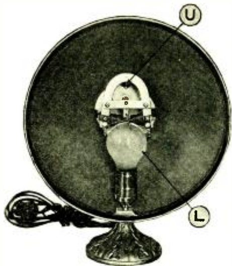
Inside view of "glow" speaker, showing method of mounting electric lamp (L) and loud speaker unit (U).
