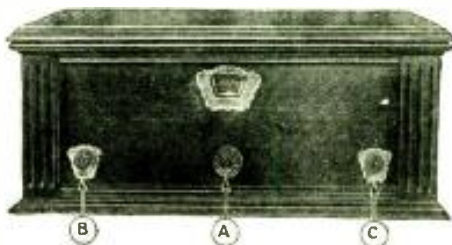
Illustrations courtesy Stewart-Warner Speedometer Corp. Front view of receiver shows arrangement of controls on front panel. A, wavelength control; B, sensitivity control; C, volume control.
