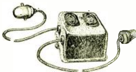
Sketch shows appearance of a simple power switch which may be used for controlling operation of both "A" and "B" power units.
