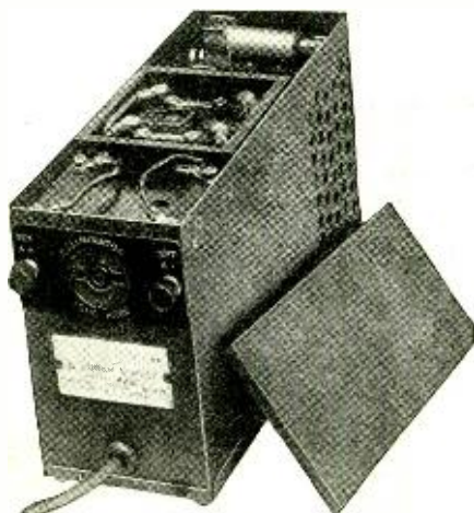
Fig. 8. A typical "A"-power-supply unit, using the new rectifier, along with a small storage battery.
