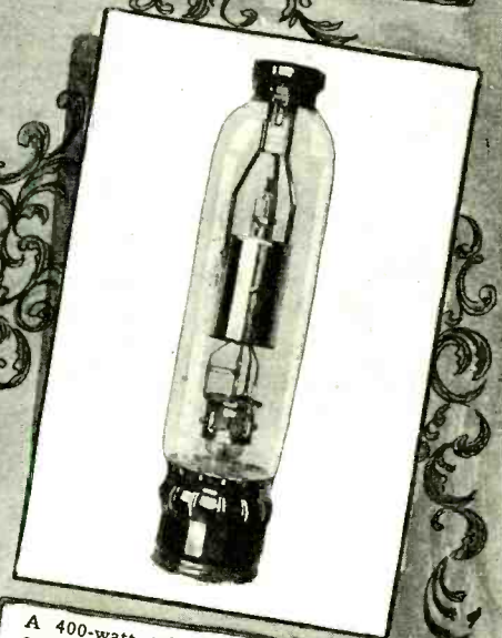
A 400-watt tube, used to supply the constant-carrier wave in the first stage of the transmitter. It uses 12 amperes at 22 volts "A" current, and 2,000 volts "B."
