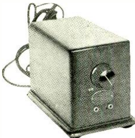
The wooden case of the amplifier is finished in walnut, and presents a pleasing appearance. The knob, actuating the shaft of the 500,000-ohm potentiometer, acts as a combined volume control and filament switch. The two small jacks at the bottom accommodate the loud-speaker tips.
