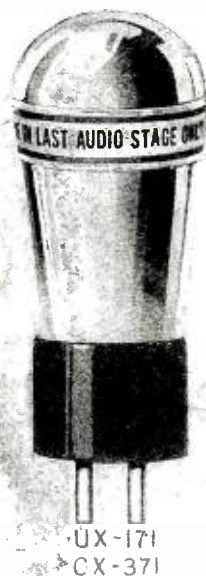
A new storage-battery type power amplifier tube, for use in the last stage audio amplifier only. This tube takes the same filament voltage and filament current as the No. 112 tube shown above, but employs a "B" voltage of 180 and a 40½-volt "C" battery. Special means should be provided for handling its heavy output. Two arrangements are shown in Fig. 6.
