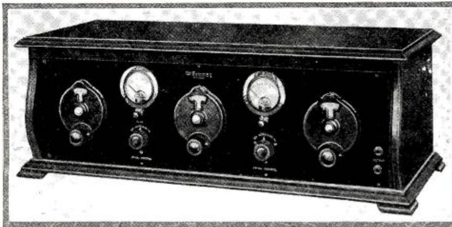
The panel of this super-heterodyne is symmetrical and the meters show the conditions which should be known.
