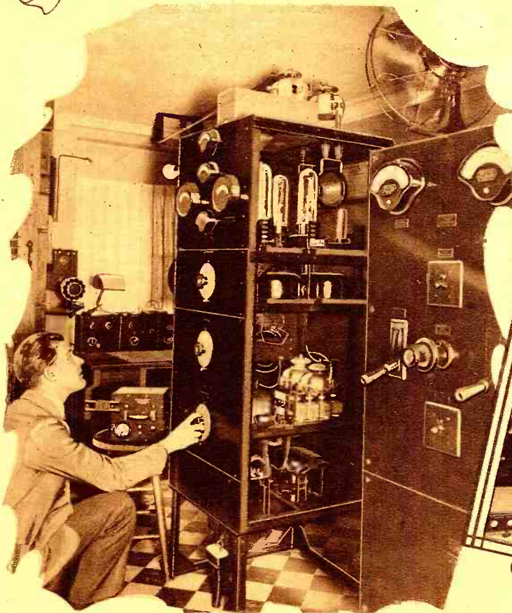
THE TRANSMITTER AND CONTROL PANELS. In the transmitter can be seen the large tubes and tuning apparatus and on the right is the panel on which is mounted the apparatus which controls the motor generator set.
