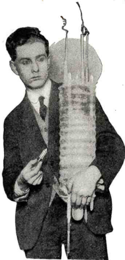
A baby and a giant. The large transmitting tube is made of Silica and is rated at 30 K.W. The filament draws 50 amperes at 30 volts. The plate voltage is 12,000. The little tube is employed as detector or amplifier. The filament draws 0.25 amperes at 1.1 volts.
