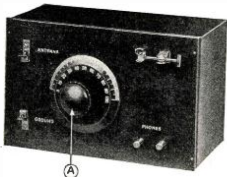
Fig. 3. An elementary type of receiver using a crystal detector is illustrated above. A is the tuning control.
