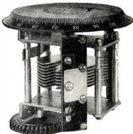
The condensers used in the complete set are set vertically with dials and verniers which protrude through the cabinet at right angles to the panel.
