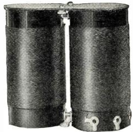
Fig. 8. A photograph of the complete binocular coil is shown above. Note the size of the tubes and the Litz. winding.
