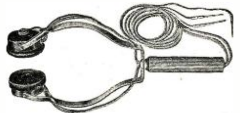
A headset, made especially for listeners of the gentler sex, is mounted on a hollow, wooden handle. With this pair of phones Milady need not fear that her coiffure will be disarranged, due to the old style head set, while she is listening-in.
