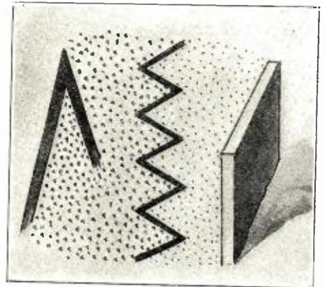
How the grid, when negative, actually impedes the electron stream generated by the hot filament is clearly shown in the above illustration.
