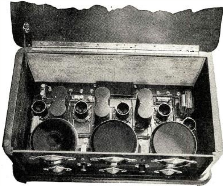
The completed set described in this article is shown in the photograph at the left. The large discs at the front of the set are the dials of the condensers which are placed vertical to the panel front. The binocular coils, radio frequency transformers, are plainly visible between the sockets. Photos © 1925 by A. H. Grebe & Co., Inc.
