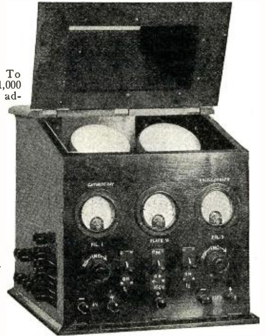
The white disks are the ends of oscillograph tubes on which the frequency patterns appear.
