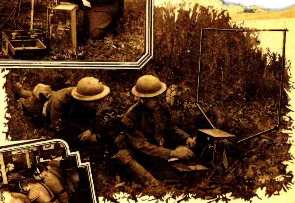
A PORTABLE FIELD SET. This signal corp sergeant saw service in France with the first division and knows a good shell hole when he sees one. It took him but two minutes to erect this battalion radio set; it was carried by two men, and establishes communication with a division set. This is all a part of the day's work at the Signal Corps School for the army at Camp Vail. (By United.)
