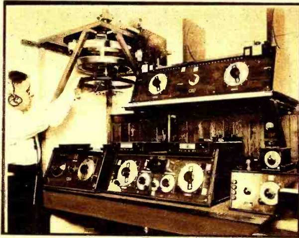
GERMAN RECEIVER (above). A view of the receiving apparatus in the large station at Geltow, Germany, where messages from the United States are received every day. Note the operator setting the loop aerial. © The Gilliams Service, N. Y.
