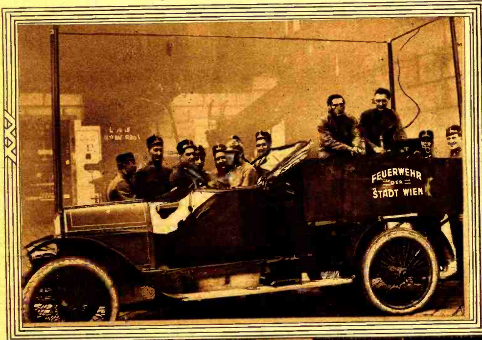
(Above) One of the Vienna fire-prevention automobiles equipped with radio transmitting and receiving apparatus. Note the antenna, strung on the four poles attached to the front and rear of the car. Right: Anton Wagner, head of the Vienna Fire Department, listening in on the headquarter's radio receiving set.
