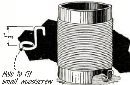
A coil clamp easily made.
