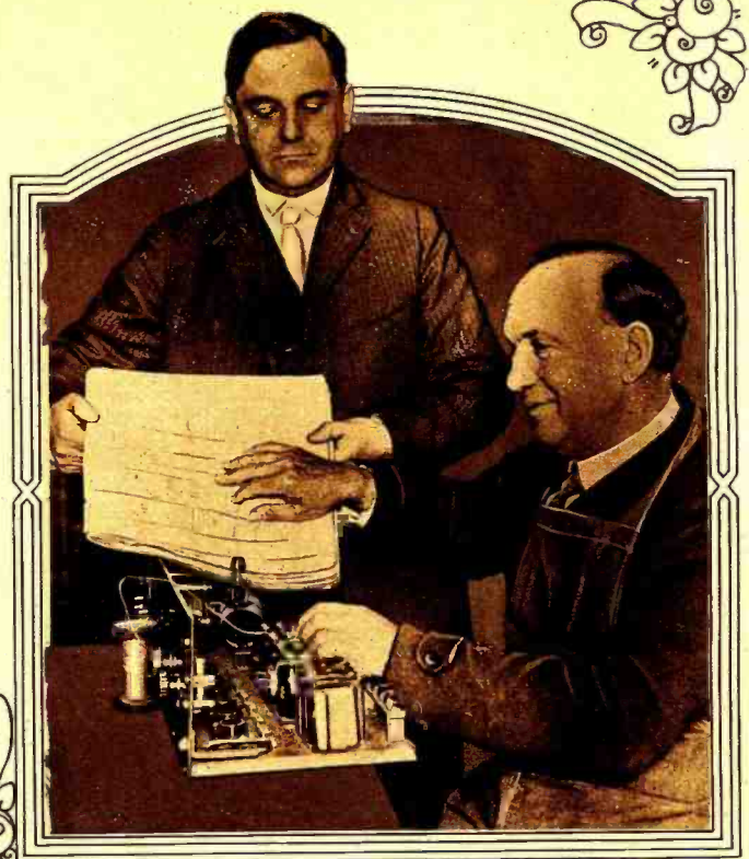
THOUGH BLIND , Harry Scott, shown in the photograph above, built his own radio set. He followed a new Braille system blue print of the circuit connections, feeling out each raised line on the print and placing the wire in the set in accordance with the circuit. © Kadel & Herbert.
