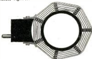
Minimum insulation reduces losses in this coil.
