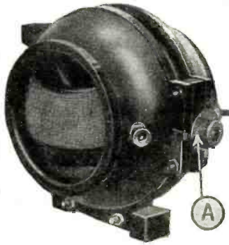
Fig. 11. The variometer also has pigtail connections which sometimes get out of order.
