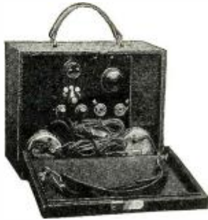
Model P-12 Two-tube Portable. (Model P-11 with amplifying tube added, which increases distance and volume many times.)
