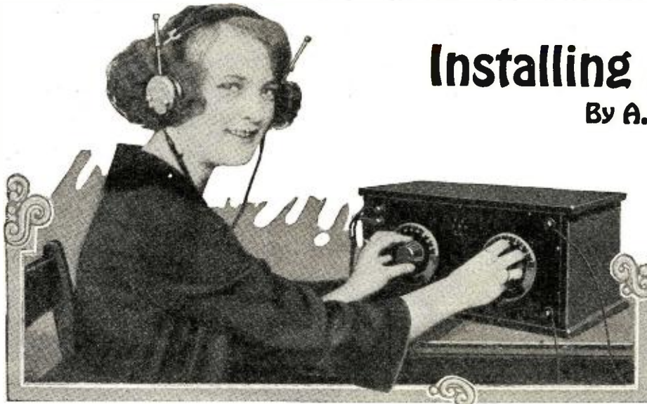
Fig. 10. Operating a two control regenerative vacuum tube receiving set. The left knob and dial is employed to tune with, while the right knob and dial controls regeneration.
