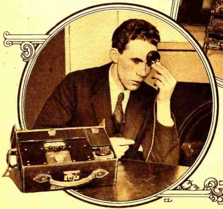
RADIO FOR THE DEAF has been made possible by this new device shown at the recent Medical Exhibition at Westminster, in England. The set is of ordinary type, employing two vacuum tubes. The contact device, which takes the place of the usual headphones, when placed against the elbow, knee or forehead, faithfully imparts the vibrations to the bones of the listener, which in turn affect the auditory nerves. It has been stated that a lady visitor to the Exhibition, who had not heard for 40 years, was able to hear music through the medium of this instrument.
