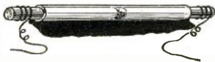
Leading to the first electrolytic detector was a glass tube with two metal electrodes with a paste or glycerine and water between them.
