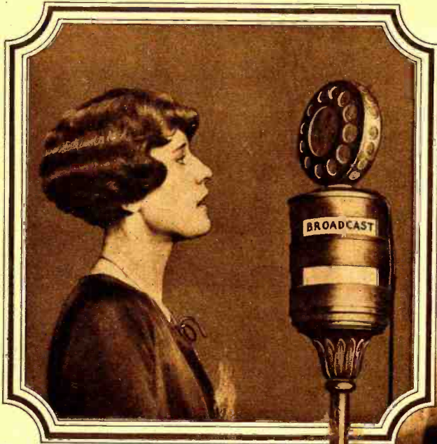
"PREPARE-BROADCAST" says this microphone to the artist and is perfectly silent. Beneath the regulation microphone is an electric sign that does the informing. It is controlled by the studio announcer. © United.
