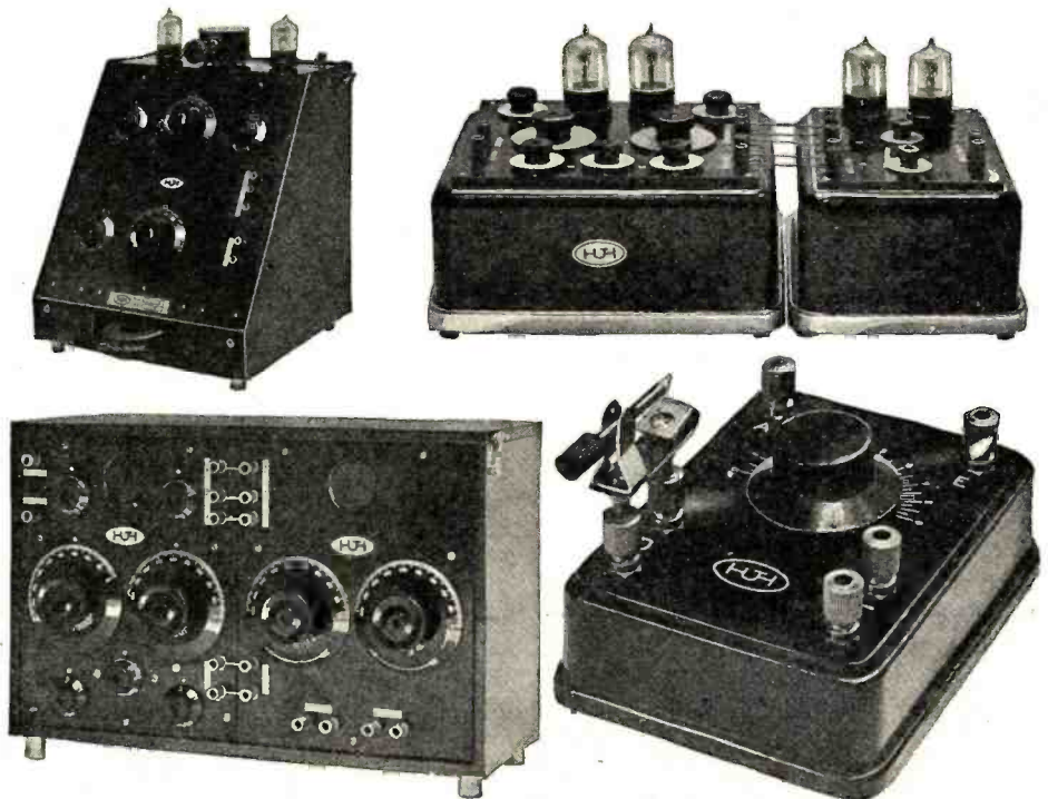
A few late models of radio receiving sets of German manufacture recently exhibited. The set in the lower left hand corner shows ear marks of American design. Note the binding posts employed on the sets; they are combination posts and jacks.
