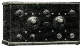
Model C-13 Three-tube Receiver. Gives five-tube volume with only three tubes, due to reflex amplification.
