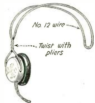
When an extra head-band is needed, it can be made in a few minutes with heavy wire.
