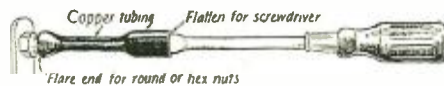
Handy socket wrenches can be made from a piece of copper tubing in the manner shown.
