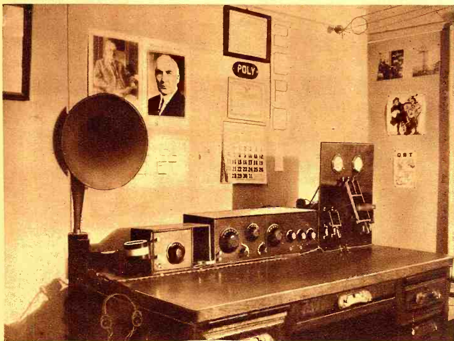
Station 2CPQ, owned and operated by John C. Phipps, Brooklyn, N. Y. The transmitter employs a 50 watter in a Hartley tuned counterpoise-ground circuit. Plate current is secured from an Acme 200 watt transformer. The receiver is of the three circuit type and covers wave bands of 150 to 415 meters and 290 to 825 meters. 2CPQ has been heard in 23 States and Canada.
