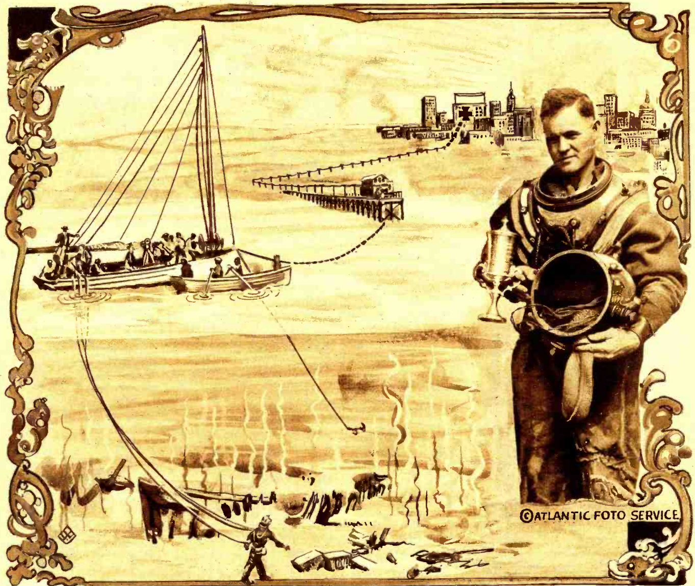
Mr. G. A. Jackson, the deep sea diver, after having broadcast his experiences in "Davy Jones' Locker," and the silver loving cup presented to him by Miss Alma Tell, noted actress. The accompanying sketch shows how Jackson's voice was carried in the form of an electric current, from his helmet to the boat, from the boat to the pier and thence to broadcast station WIP by telephone, from where it was transmitted into the ether to be heard by listening radio fans.
