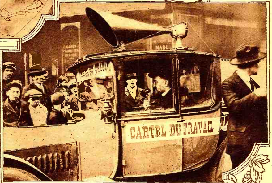
During the last political campaign in France the contestants in the elections did their campaigning in de luxe fashion. At the right is shown a candidate with his car and loud speaker. His voice was spoken into a microphone and passed through an audio amplifier from which it was delivered to the horn atop the car which he used in traveling about his district. P. & A. Photos.
