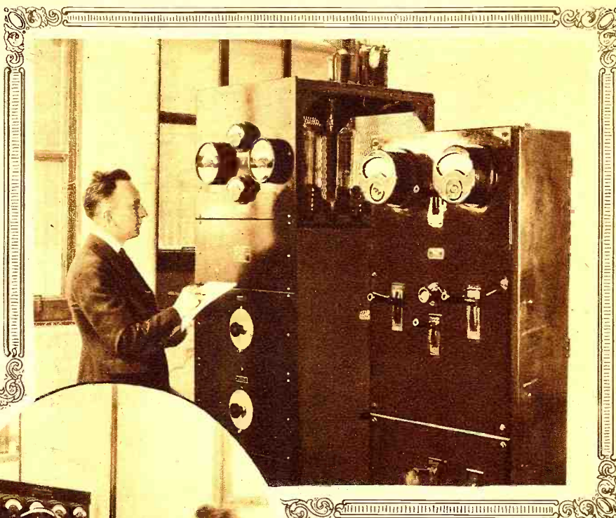
A Typical Radiophone Transmitter. On the Right is the Control Panel and on the Left the Transmitter Proper.
