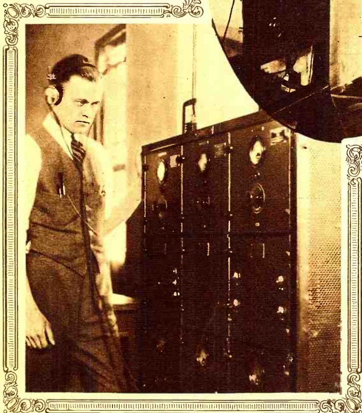
These Two Pictures Show the Type of Amplifiers Through Which the Voice and Music Are Amplified Before Reaching the Transmitter. An Operator Listens Constantly to Check the Quality and Volume. © Photoneus
