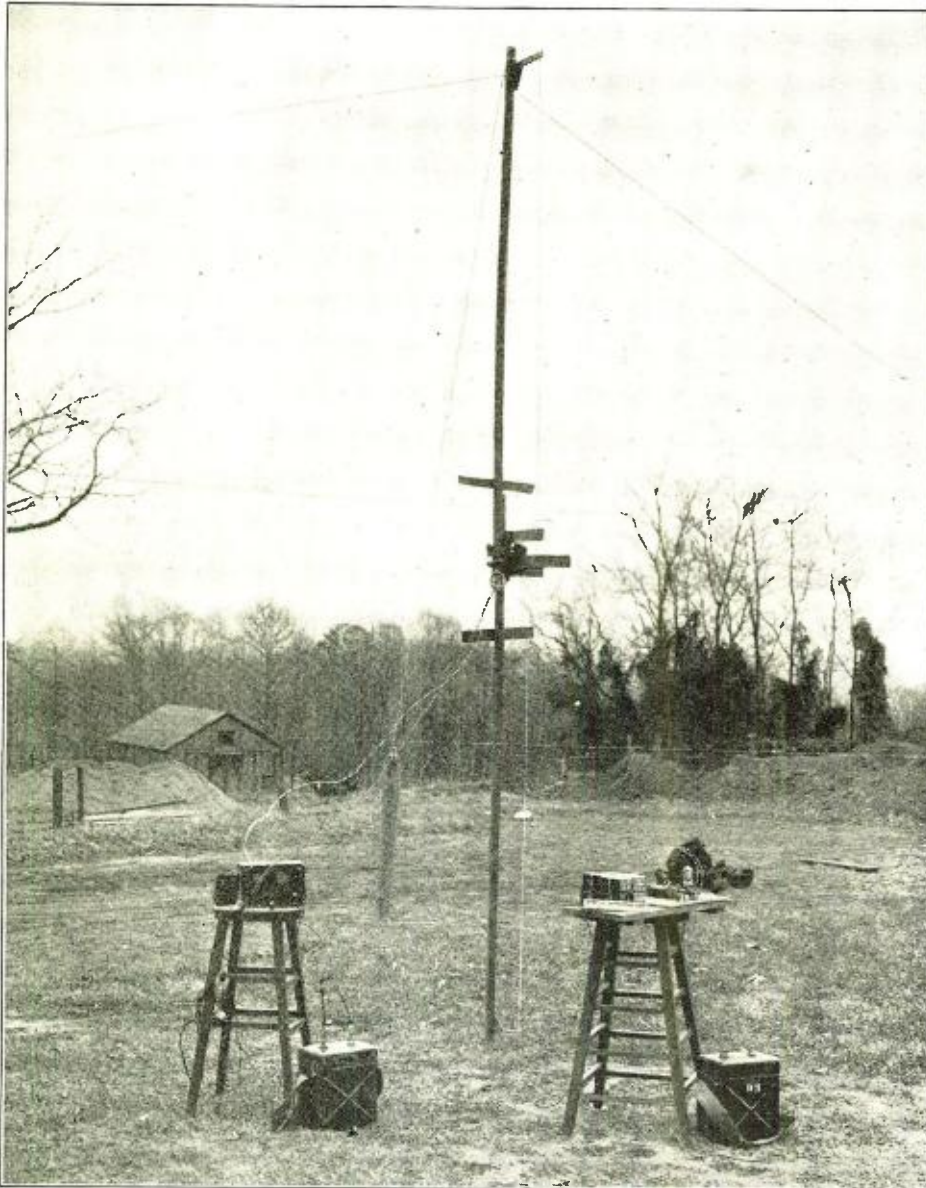
Fig. 7. Ten-Meter Receiving Set. Note on the Mast the Single Turn Coupler and Detector Tube. The Amplifier May Be Seen on the Left Stool and the Heterodyne on the Right One.
