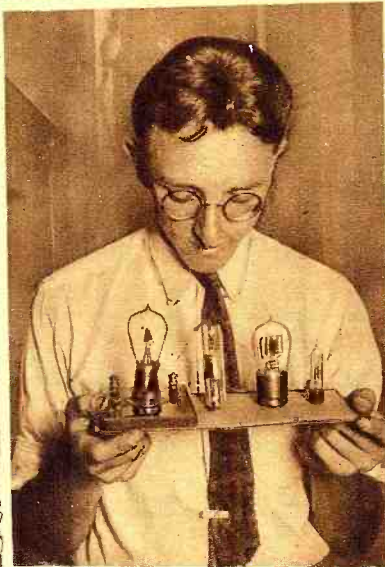
Great Strides Have Been Taken, Particularly in the Design of Vacuum Tubes. The Board Held by the Man Includes, First, the Fleming Two-Element Vacuum Tube Followed by a Three-Element Audiotron, a Radiotron and, Finally, One of the Latest Types of "Peanut Tubes." Further On We Have Three Large Transmitting Tubes of the Type Used Today. The First One Is Of One Hundred Kilowatts Capacity and Two of These Can Do the Same Amount of Work as the Giant Alternator Pictured Directly Above. Note Its Size In Comparison With the Peanut Tube In the Same Photo
