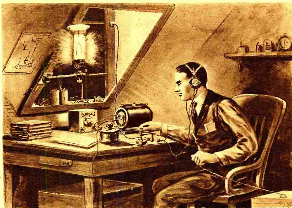
While Experimenting With a New Detector in 1900, Dr. de Forest Discovered That the Light of a Gas Burner Was Affected by the Discharges Produced by a Spark Coil.
