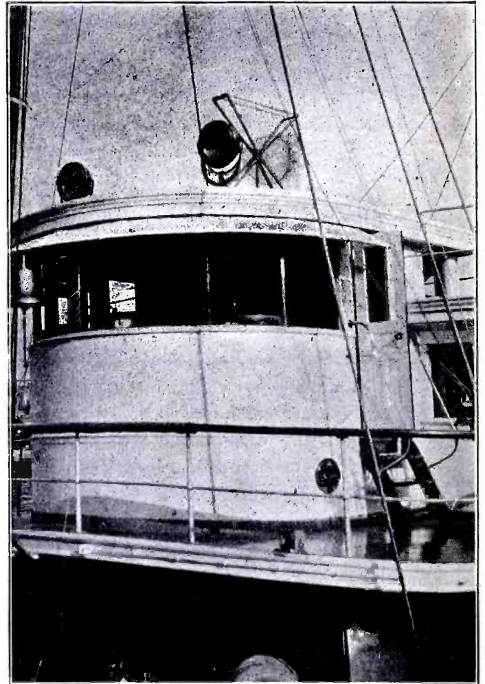
The Pilot House of the "Tulip", on Which May Be Seen the Loop Aerial of the Compass Set.
