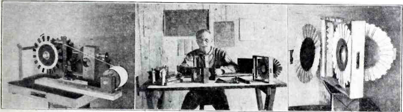
Three Photographs Taken at Radio Hill. To the Left We Have a Practical Working Model Devised by the Inventor for the Purpose of Rapidly Winding "Spider Web" Coils. In the Center Is Shown Mr. Eugene T. Turney, a Practical Idealist, Surrounded by Some of His "Pets" While to the Right Is a Long-Wave Three-Coil Receiving Unit Consisting of Primary, Secondary and Tickler, the Primary and Tickler Being Variable in Respect to the Secondary in the Center.
