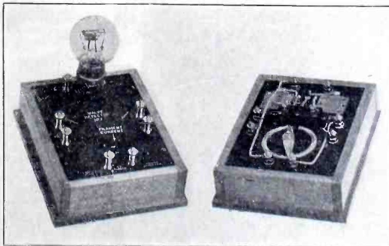
To the Left of This Illustration is Shown the Instrument With Vacuum Tube Ready for Use While to the Right We Have the Base turned In Such Manner as to Show Internal Set-Up.
