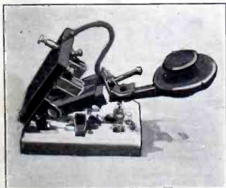
Here is the Actual Model of the Two-in-One Aerial Switch-Sending Key Which Mr. Clark Designed.
