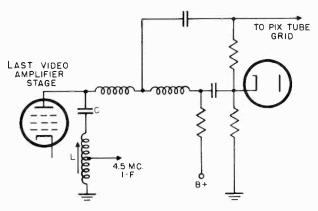
Figure 45. Circuit used to separate the sound carrier from the video signal in intercarrier receiver.
