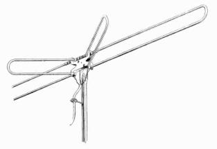
Figure 39. Bat-wing antenna.
