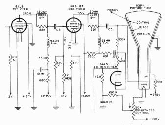
Figure 65. Two stage video amplifier suing shunt and series peaking.
