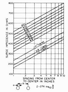
Figure 18. Characteristic impedance of two-conductor parallel transmission lines.
