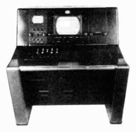
Figure 35. Picture monitor. (courtesy DuMont)
