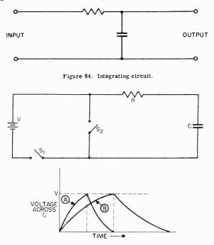
Figure 85. Operation of integrating circuit.
