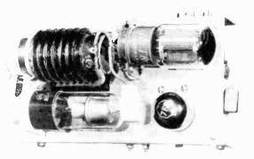
Figure 151. Pulse type power supply.
