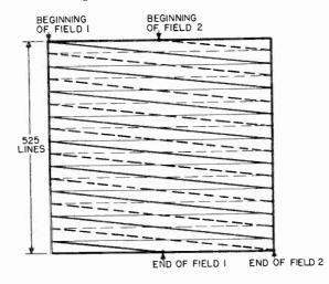
Figure 53B Interlaced scanning pattern.
