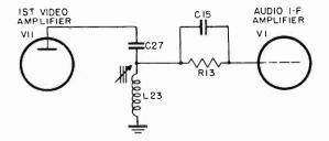
Figure 17. Coupling circuit for separating video and audio signals.
