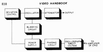
Figure 9. Block diagram of fundamental frequency wobbulator.
