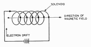
Figure 24. Direction of magnetic field in a solenoid.
