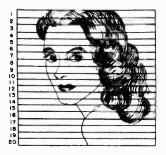
Figure 9. How linear scanning is accomplished.
