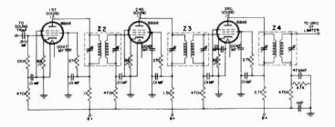
Figure 164. Three-stage sound i-f amplifier.
