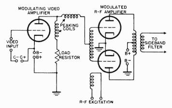
Figure 52. Modulated Class B amplifier,
