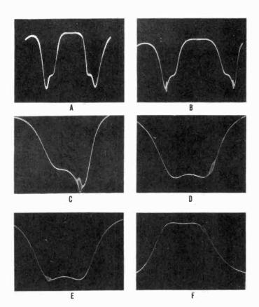
Figure 72. Fesponse curves obtained when aligning video i-f amplifiers. A. Dual response curve, B. Birdie at 26.4 Mc, C. Single response curve, D. Birdie 1 db down from flat top, E. Birdie at 22.4 Mc, F. Birdie at 26.4 Mc.
