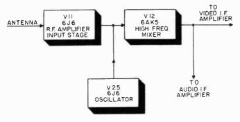
Figure 11. Block diagram of DuMont Inputuner.
