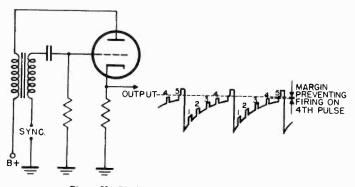
Figure 23. Blocking oscillator frequency divider.
