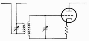
Figure 29. Antenna coupling circuit using tuned primary and secondary.
