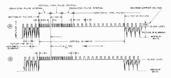
Figure 19. Standard F.C.C. television signal.
