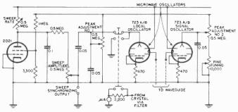
Figure 15. Basic schematic circuit of Mega-Sweep.
