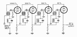
Figure 26. Frequency divider chain.
