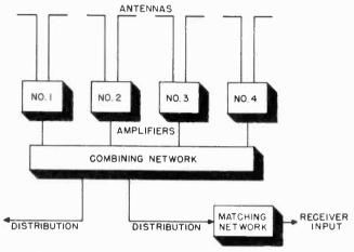
Figure 84. Block diagram of Intra-Video master antenna system.
