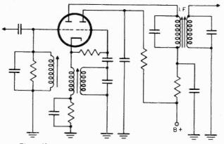
Figure 18. Mixer-oscillator using dual triode with common cathode.
