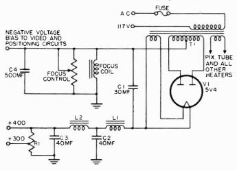
Figure 143. Typical low-voltage power supply.
