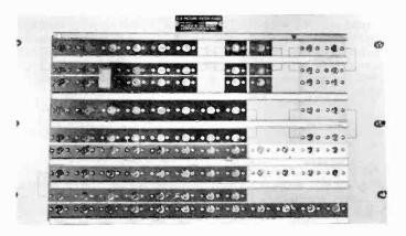
Figure 67. On-the-Air patch panel. (courtesy DuMont)
