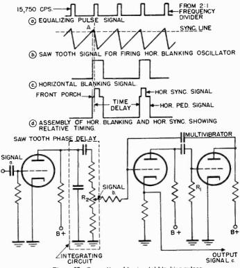
Figure 27. Generation of horizontal blanking pulses.
