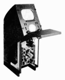
Figure 90: Studio picture monitor. (courtesy RCA)
