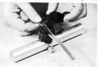
Figure 31. Lightning arrestor. (courtesy RCA)
