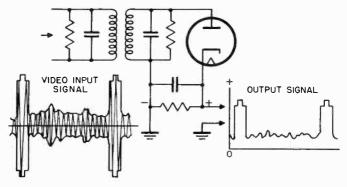
Figure 53. Diode detector and waveform.
