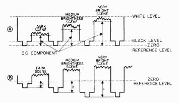
Figure 70. A, video signals of three different screen brightness levels. B, video signals with d-c component removed.
