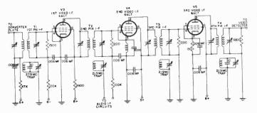
Figure 50. Overcoupled i-f amplifier with wavetraps.
