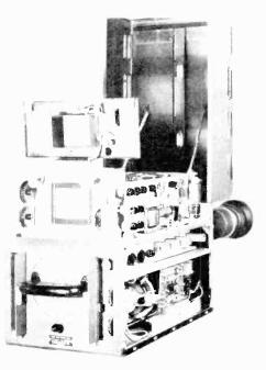
Figure 14. Pickup head and electronic viewfinder. (courtesy DuMont)
