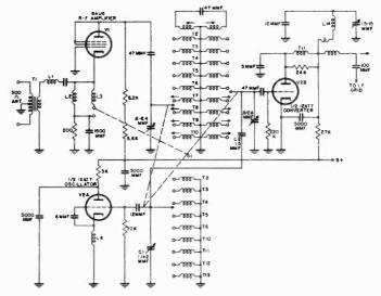
Figure 4. Schematic diagram of G.E. tuner.
