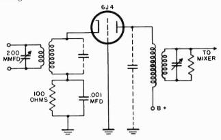
Figure 6. Grounded-grid r-f amplifier.
