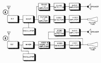
Figure 43. Block diagrams of receivers using conventional and intercarrier sound systems.
