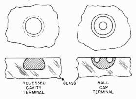
Figure 125. Intensifier terminals.
