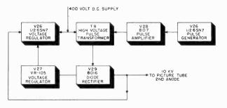
Figure 41. Block diagram of 10KV high voltage supply.
