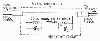
Figure 40. Circuit for wave trap.
