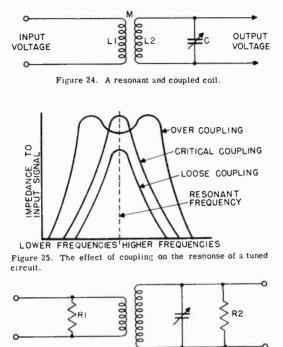
Figure 26. Transformer shunted with resistors to flatten and broaden its response.
