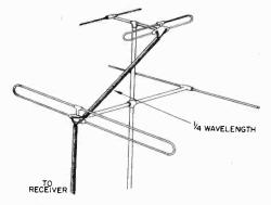
Figure 45. Antennas connected in parallel.
