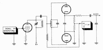
Figure 62. Connections used when checking limiter performance.
