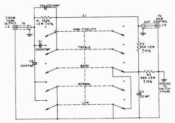
Figure 47. Tone selector schematic.
