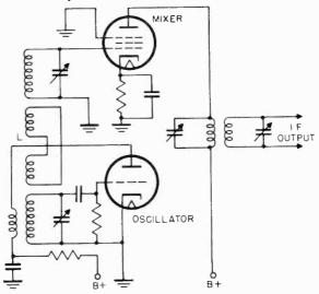
Figure 15. Inductively-coupled mixer-oscillator,
