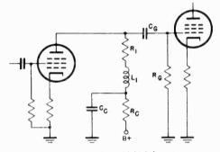
Figure 2. Oscillograph amplifier with high frequency compensation.
