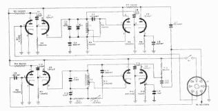
Figure 18. Schematic circuit of Crosshatch Generator
