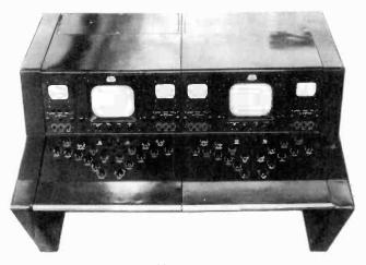
Figure 97. Iconoscope film camera monitor showing shading controls. (courtesy DuMont)
