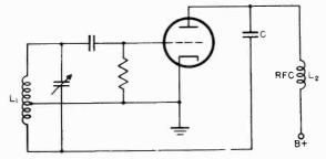
Figure 9. Shunt-fed Hartley oscillator.
