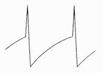
Figure 150. Pulses generated by blocking oscillator.
