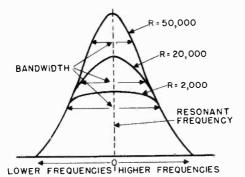
Figure 27. The effect of various values of load resistance on bandwidth of coupling transformers.
