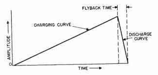
Figure 32. A sawtooth voltage.
