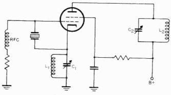
Figure 44. Tri-tet oscillator.
