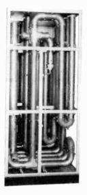
Figure 110. Vestigial sideband filter. (courtesy RCA)
