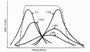
Figure 54. Relative gain and selectivity of each coil in staggered i-f amplifier. Resulting overall response curve is shown dotted in background.
