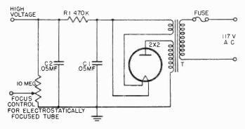
Figure 145. Circuit of a 60-cycle, high-voltage supply.
