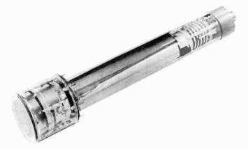
Figure 5. The image orthicon. (courtesy RCA)
