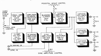
Figure 37. Block diagram of mixing and distribution amplifier.
