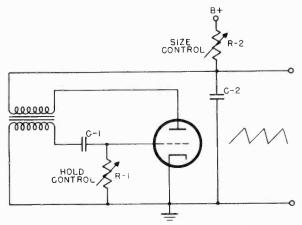
Figure 109. Blocking oscillator and discharge circuit.
