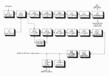
Figure 43. Block diagram of r-f, i-f chassis.
