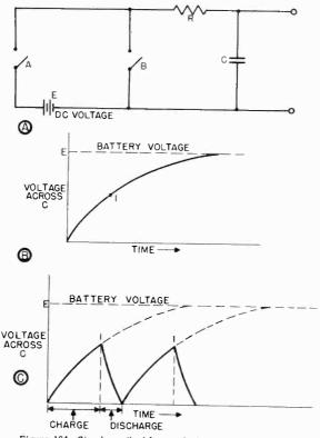
Figure 104. Simple method for producing saw-tooth voltage.
