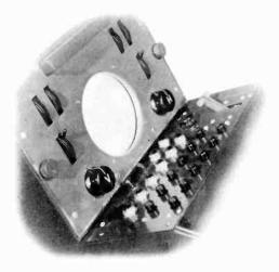
Figure 91. Camera switching monitor controls. (courtesy RCA)
