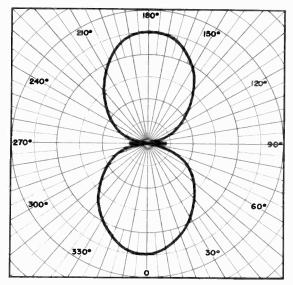
Figure 40. Field pattern of bat-wing antenna at 80 Mc.
