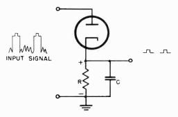
Figure 81. Self-biased diode sync clipper.
