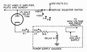
Figure 40. Automatic, high-voltage cutoff circuit.
