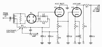
Figure 76. Delayed a.g.c. circuit.
