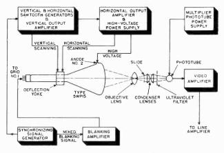
Figure 101. Block diagram of flying spot signal generator.
