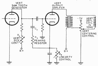
Figure 117. Vertical amplifier circuit.
