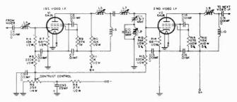
Figure 77. Gain control by varying the grid bias on remote cutoff pentode i-f amplifiers.
