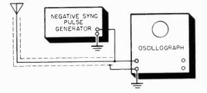
Figure 130. Method used to check antenna impedance match.
