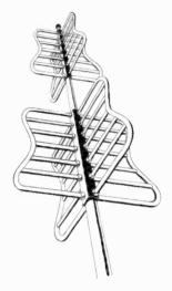
Figure 78. Super-turnstile antenna.
