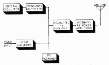
Figure 43. Block diagram of low level modulated transmitter.
