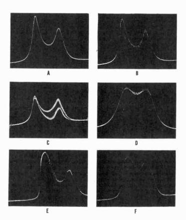
Figure 64. Response curves of sound i-f amplifiers. A. Single i-f response curve, B. Response curve with birdie at 21.9 Mc, C. Effect of too much birdie, D. Response curve of properly aligned i-f amplifier, E. Effect produced by slight overload, F. Effect produced by excessive overload.
