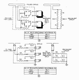
Figure 87. Simple master antenna system.
