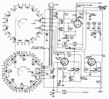
Figure 5. Schematic diagram of the Philco tuner.
