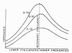
Figure 23. The effect of  ${\bf Q}$  on the selectivity of a parallel tuned circuit.
