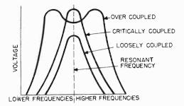
Figure 38. Effect of coupling on the response of a tuned circuit.
