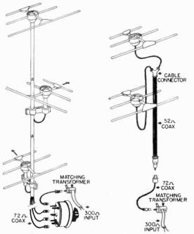
Figure 44. Typical application of coaxial switch.
