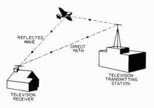
Figure 8. Reflected wave caused by moving airplane.
