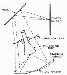
Figure 136. Light from a single point on the picture tube screen passes through all points of the corrector lens.
