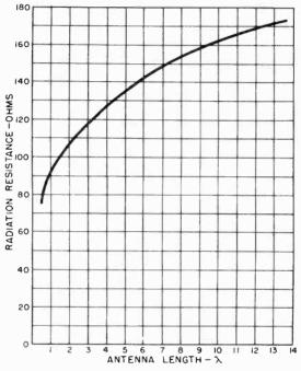
Figure 73. Radiation resistance of long-wire antenna.
