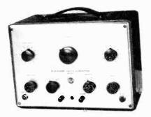
Figure 13. RCA WR-59A Television Sweep Generator.
