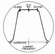
Figure 163. Response curve of a broadband i-f amplifier.
