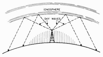
Figure 2. The two principal modes of wave propagation.
