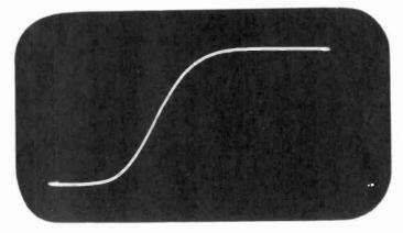
Figure 124. Leading edge of horizontal pulse.
