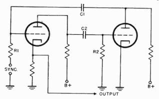
Figure 22. Multivibrator frequency divider.
