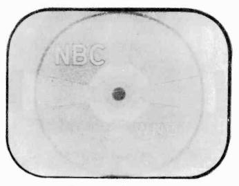
Figure 67A Insufficient contrast.
