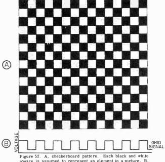
square is assumed to represent an element in a picture. B, grid voltage which is required to produce checkerboard pattern on the screen of the picture tube.
