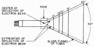
Figure 132. Relative sizes of magnetic picture tubes.
