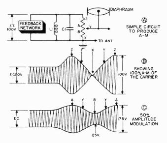
Figure 157. Simple method of amplitude modulation.
