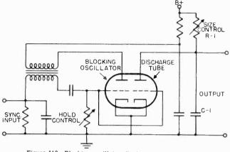
Figure 110. Blocking oscillator discharge circuit using dual triode.
