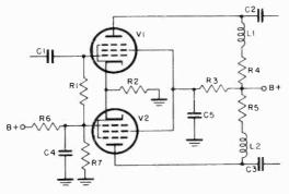
Figure 4. Cathode-coupled output stage.
