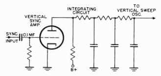
Figure 87. Cascaded integrating circuit.
