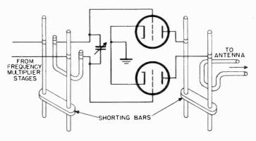
Figure 46. Transmission line tuned push-pull r-f amplifier stage.
