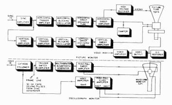
Figure 36. Block diagram of picture and oscillograph monitor.
