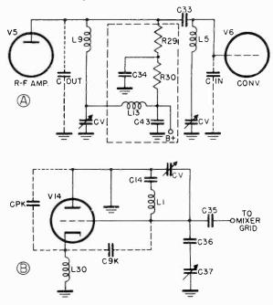
Figure 9. A. R-F amplifier circuit. B. Oscillator circuit.
