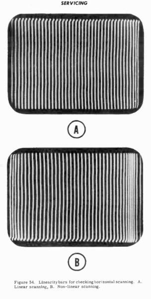
Another cause of non-linearity is the failure of a component in the horizontal deflection circuit, as for example a defective charging resistor or capacitor in the sawtooth generator circuit, or a faulty sweep-amplifier tube. Such faults should be isolated by signal tracing the entire sweep circuit and comparing the waveforms with those shown in the manufacturer's service manual.
