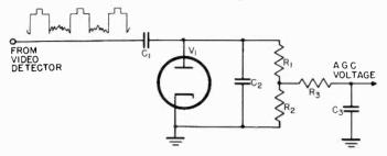
Figure 75. Simplified diagram of a.g.c. circuit.
