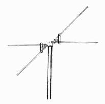
Figure 42. Double-V antenna.
