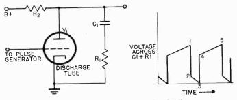
Figure 115. Discharge tube with peaking circuit.
