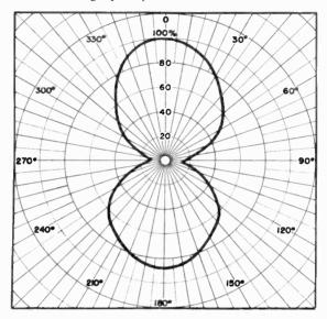
Figure 37. Horizontal field pattern of duo-dipole antenna at 70  $\mbox{Mc}.$
