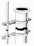
Figure 20. Bracket for mounting on vent pipe.
