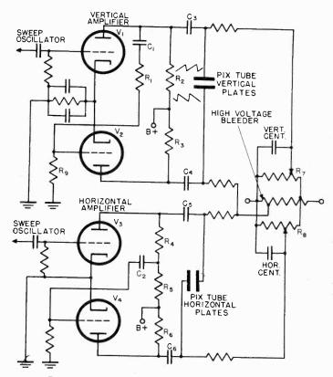
Figure 113. Push-pull vertical and horizontal sync circuits for electrostatic deflection.
