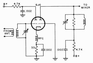
Figure 7. Cathode-coupled r-f amplifier.
