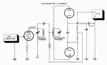
Figure 56. Connections used when aligning discriminator using v.t.v.m.
