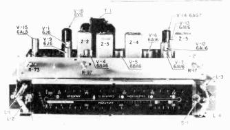
Figure 44. R-F, I-F chassis showing slide-rule dial. (courtesy DuMont)
