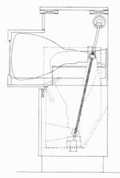
Figure 127. Mechanical lift mechanism used with large picture tubes.
