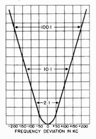
Figure 162. Typical i-f amplifier response curve.
