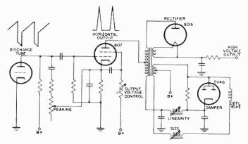
Figure 153. Simplified schematic of kickback high-voltage supply.
