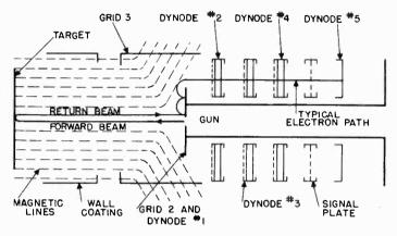
Figure 10. Electron Multiplier Section of the image orthicon.
