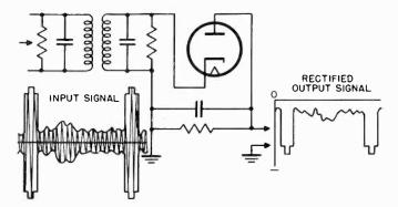
Figure 56. Diode detector and waveform.
