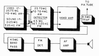
Figure 44. Operation of the intercarrier sound system.
