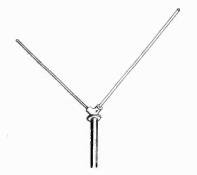
Figure 31. Adjustable V antenna.
