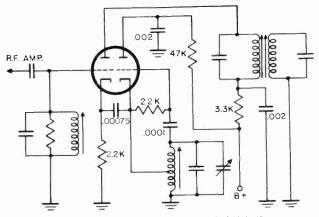
Figure 16. Mixer-oscillator using cathode injection.
