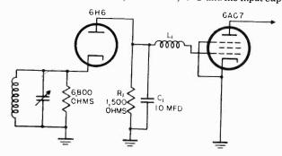
Figure 58. Direct coupled video detector.
