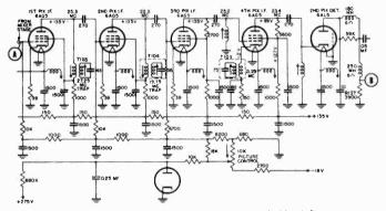
Figure 74. Schematic diagram of stagger-tuned video i-f amplifier.
