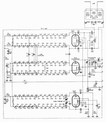
Figure 2. Schematic diagram of RCA tuner.
