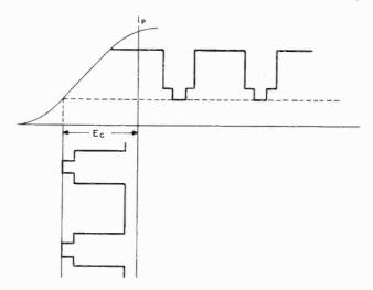
Figure 53. Grid characteristic of Class B modulated amplifier.
