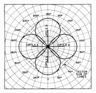
Figure 34. Horizontal field pattern of crossed dipole antenna.
