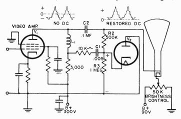
Figure 71. Schematic of diode d-c restorer.
