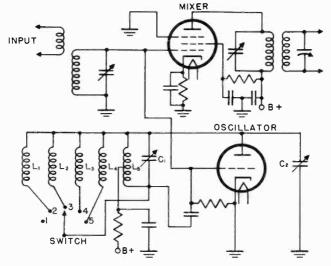
Figure 11. Hartley oscillator for covering widely separated frequencies.
