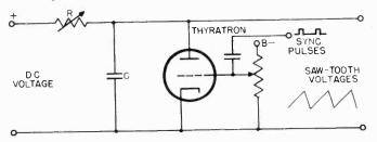
Figure 107. Thyratron saw-tooth generator circuit.
