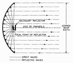
Figure 80. Reflecting action of parabolic surface.
