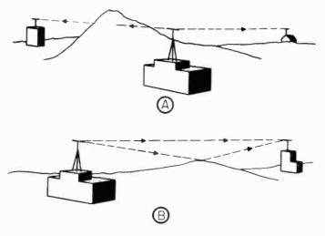
Figure 10. (A) Television signal weakened by intervening hill. (B) Multipath reflection caused by a "bounce" signal.
