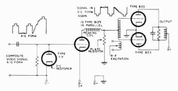
Figure 56. D-C reinsertion in grid circuit of video modulator
