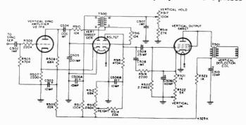
Figure 25. Vertical-deflection circuits.
