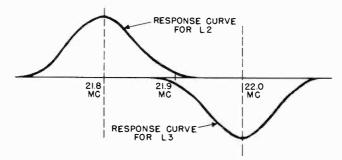
Figure 171. Response curve of tuned circuits of discriminator.
