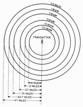
Figure 4. Ground-wave signal range of television station.
