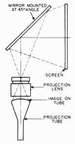
Figure 133. Refractive projection system.
