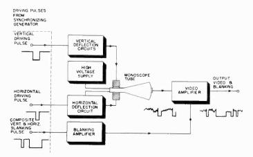
Figure 100. Block diagram of monoscope camera circuit.
