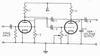
Figure 96. Multivibration circuit.
