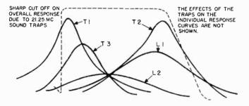
Figure 42. Response curves of stagger tuned i-f amplifier.
