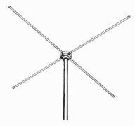
Figure 33. Crossed dipole antenna.
