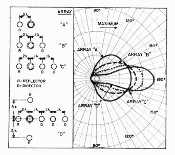
Figure 56. Field patterns of four parasitic arrays.
