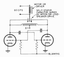
Figure 10. Variable capacitor circuit for wobbulator.
