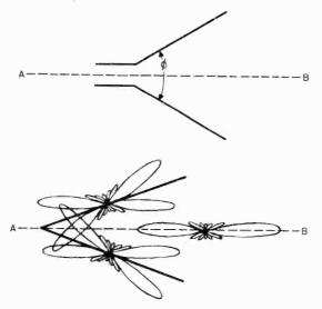
Figure 74. V antenna, and method whereby field patterns of two long-wire radiators are combined to produce highly directional V antenna field pattern.
