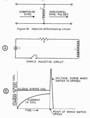
Figure 90. Operation of inductive differentiating circuit.
