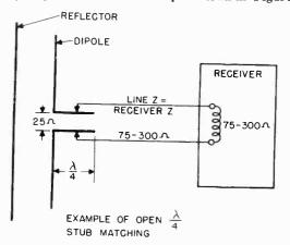
Figure 23. Quarter-wave stub matching section.
