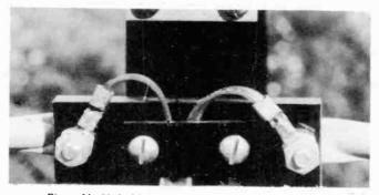
Figure 14. Method for connecting twin-lead to antenna. (courtesy Taco)
