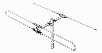
Figure 55. Folded dipole with reflector. (courtesy JFD)
