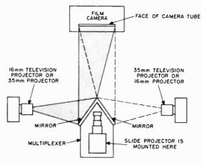
Figure 99. Physical layout of film multiplexer.
