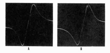
Figure 60. Signal on oscillograph produced by discriminator output. A. Marker signal at center frequency, B. Marker signal at signal peak.
