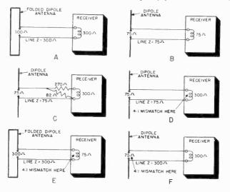
Figure 21. Examples of matched and mismatched antenna systems.
