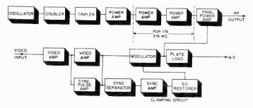
Figure 108. Block diagram of TT-5A transmitter.
