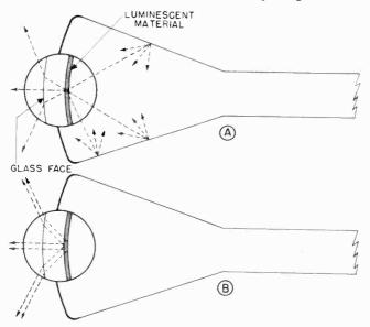
Figure 126. How aluminum backing increases image brightness.
