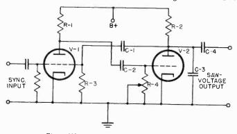
Figure 108. Multivibrator and discharge circuit.
