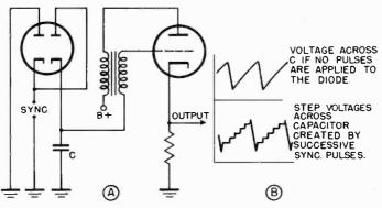
Figure 25. Pulse counting circuit.
