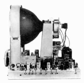
Figure 30. Main chassis of Scott Model 13-A.
