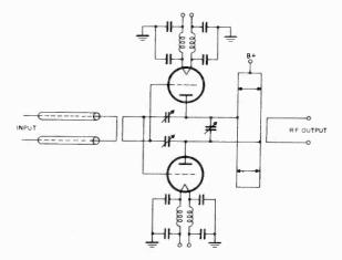
Figure 50. Wideband r-f amplifier circuit.
