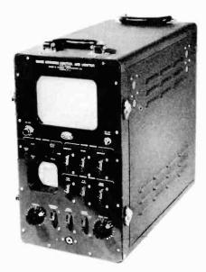
Figure 75. Camera control monitor. (courtesy DuMont)
