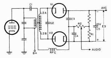
Figure 175. Simple ratio detector.
