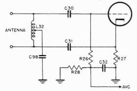
Figure 8. Antenna input circuit.
