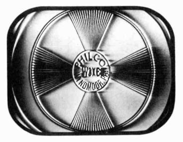
Figure 62. Test pattern showing effect of phase distortion.
