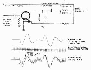
Figure 30. Forming the 60-cycle, three-line keying signal.
