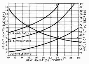
Figure 77. Design chart for rhombic antenna.
