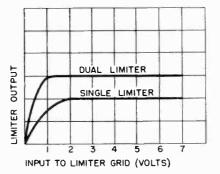
Figure 168. Comparison of single and dual limiter.
