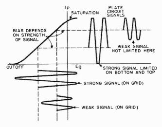
Figure 166. Operation of limiter circuit.
