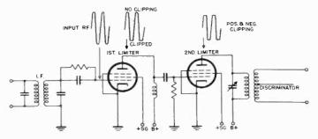
Figure 167. Dual or cascade limiter.
