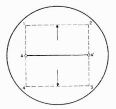
Figure 31. Raster pattern traced out by two sine waves, of equal amplitude, but of different frequency, which are applied to the vertical and horizontal deflection plates.
