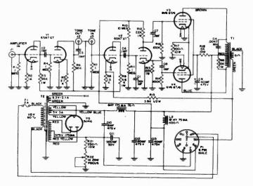
Figure 46. Audio amplifier schematic.
