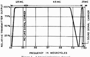
Figure 4. A typical television channel.
