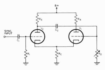
Figure 97. Cathode-coupled multivibration circuit.
