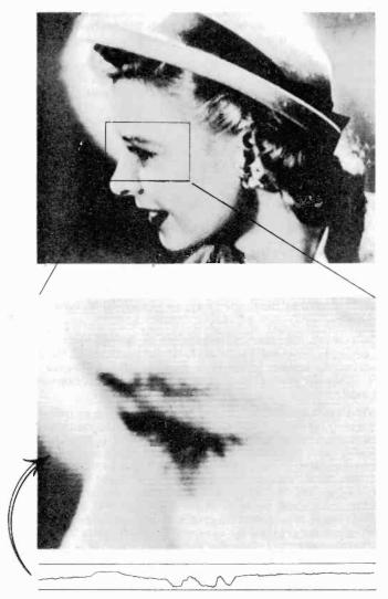
Figure 38. Grid voltage variations necessary to form one line of a picture.
