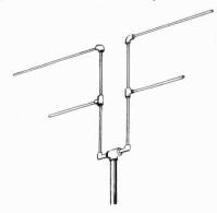
Figure 63. Stub-tuned stacked array.
