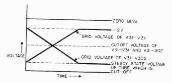
Figure 78. Curve of bias changes which occur in switching amplifiers.
