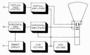
Figure 1. Block diagram of cathode-ray oscillograph.
