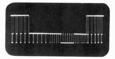
Figure 122. Vertical blanking interval. (courtesy DuMont)
