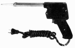
Figure 8. Soldering gun (courtesy Weller Mfg.)
