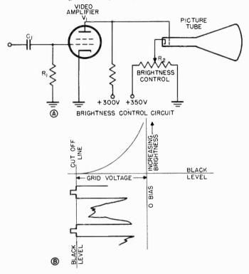
Figure 73. A, circuit for providing adjustment of picture tube blas. B, effect on picture brightness of variations in grid voltage.
