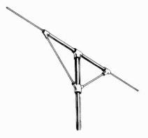
Figure 32. Extended V antenna.
