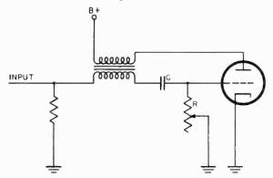
Figure 93., Blocking oscillator circuit.
