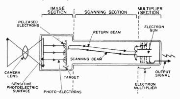
Figure 7. Construction of the image orthicon.
