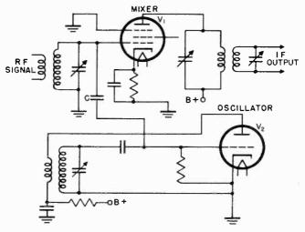
Figure 14. Capacitive-coupled mixer oscillator.
