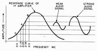
Figure 169. Operation of slope detector.
