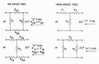
Figure 38. Attenuator network and component values.
