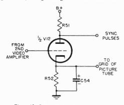
Figure 18. Sync separator and d-c restorer.
