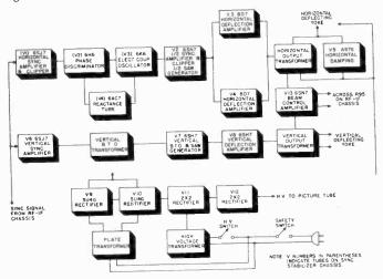
Figure 48. Block diagram of sweep chassis.
