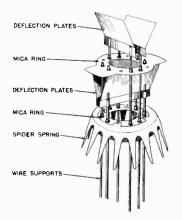
Figure 10. The deflection plate assembly.
