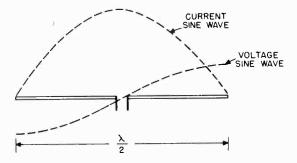
Figure 25. Current and voltage distribution on half-wave dipole.
