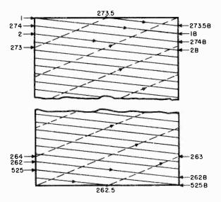
Figure 57. Method of forming interlaced scanning pattern.
