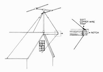
Figure 28. Outrigger used to obtain proper guy spacing.
