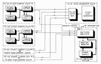
Figure 85. Block diagram of RCA studio camera equipment.
