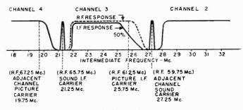
Figure 35. The relationship between the response of a television receiver, the television signal, and signals in adjacent channels.
