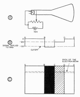
Figure 37. Forming an image on the screen.
