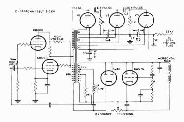
Figure 155. Kickback high-voltage supply for projection receiver.
