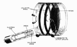
Figure 39. Construction of the Iconoscope.
