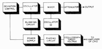
Figure 11. Block diagram of beat frequency wobbulator.
