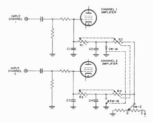
Figure 79. Simplified schematic of input switching circuits.
