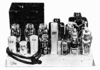
Figure 31. Power supply chassis.
