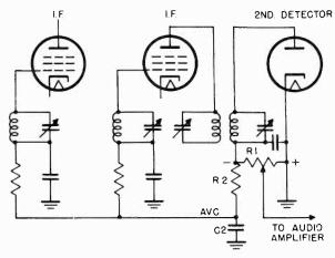
Figure 74. Simplified schematic of a.v.c. circuit of a-m receiver.
