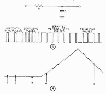
Figure 86. Input and output waveforms of integrating circuit.
