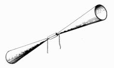
Figure 46. Conical antenna.
