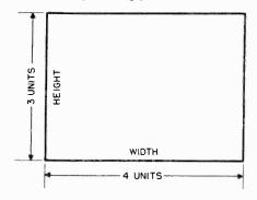
Figure 51. A pattern with a 3 x 4 aspect ratio.
