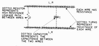
Figure 12. Distribution of resistance, capacitance, and inductance along section of two-wire transmission line,
