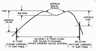
Figure 16. Response curve of intermediate frequency amplifters which pass both the video and audio signals.
