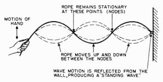
Figure 14. Standing waves produced in a rope.
