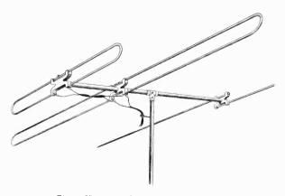
Figure 57. Duo-folded dipole parasitic array.
