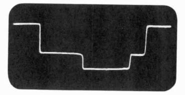
Figure 123. Horizontal blanking and sync pulse.
