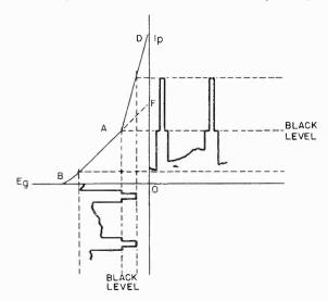
Figure 69. Grid-voltage, plate-current curves of non-linear amplifier stage.
