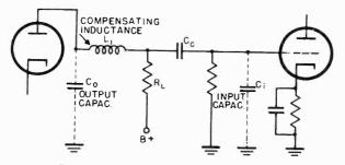
Figure 64. Series-peaking frequency compensation.
