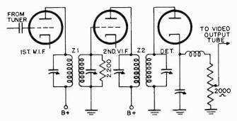
Figure 37. Simplified schematic of broadband overcoupled i-f amplifier.
