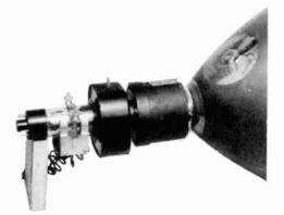
Figure 129. The ion trap magnet is mounted between the tube base and the focus coil.
