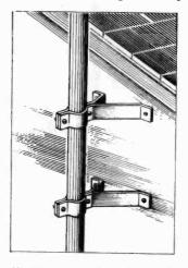
Figure 19. Wall mounting bracket. (courtesy Taco)
