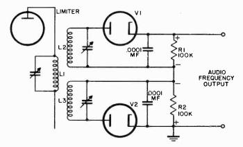
Figure 170. Simple discriminator circuit.
