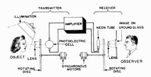
Figure 11. Transmitter and receiver apparatus for a mechanical television system.
