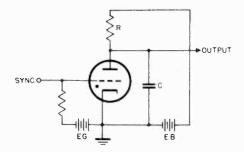
Figure 5. Gas triode sawtooth generator.
