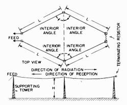
Figure 76. Rhombic antenna.
