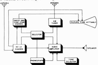
Figure 42. Block diagram of DuMont Model RA-101
