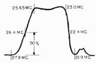
Figure 51. Response curve of i-famplifier channel using overcoupled transformer and sound traps.
