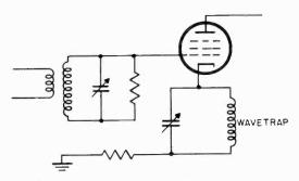
Figure 48. Simplified circuit of i-f amplifier with cathode wavetrap.
