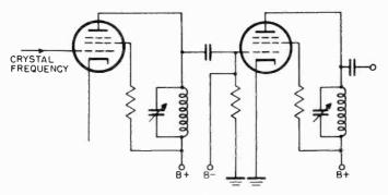
Figure 45. Simplified schematic of frequency multiplying stages.
