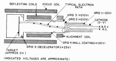
rear surface of the target. Grid 3 has little effect during the forward travel of the electron beam.
