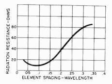
Figure 54. Variation of radiation resistance of dipole and reflector.
