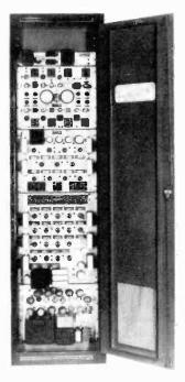
Figure 92. Studio type synchronizing generator. (courtesy DuMont)
