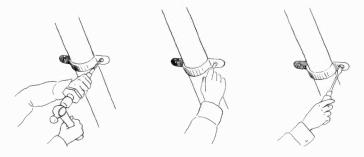
Figure 32. Drilling and mounting to masonry.
