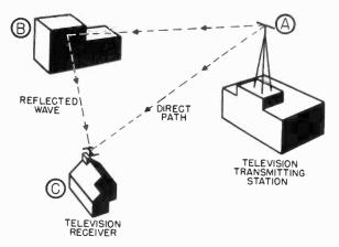
Figure 6. Direct wave and reflected wave striking antenna.
