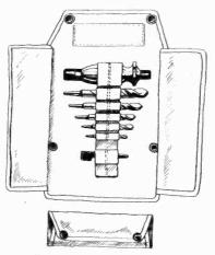
Figure 9. Masonry drill kit.
