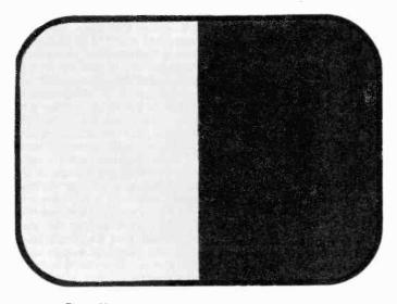
Figure 53. Pattern produced in horizontal scanning amplitude test with 15,750-cps signal on grid.
