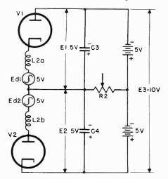
Figure 176. Equivalent circuit of ratio detector.
