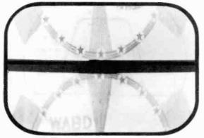
Figure 119. Test pattern with sweep set at half vertical frequency.
