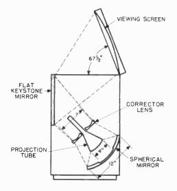
Figure 138. The Philco version of the Schmidt optical system.
