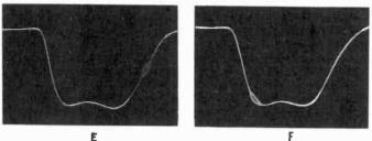
Figure 73. Response curves obtained when aligning video i-f amplifiers.
