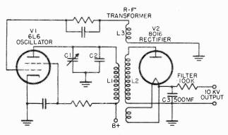
Figure 146. Circuit of an r-f high-voltage power supply.
