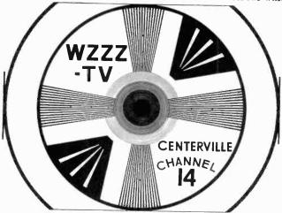
Figure 12. Pattern obtained from monoscope tube.
