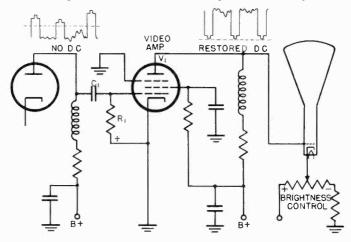
Figure 72. D-C restoration in the video amplifier stage.
