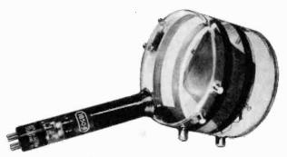
Figure 3. The Iconoscope, a cathode-ray tube used in the television camera. (courtesy RCA)
