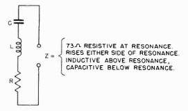
Figure 30. Equivalent circuit of a dipole antenna.
