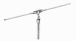
Figure 24. Dipole antenna. (courtesy Ward Products)
