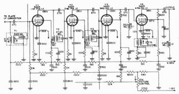
Figure 41. Stagger tuned i-f amplifier channel.
