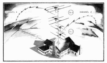
Figure 42. Multipleantenna installation using two six-element beams. (courtesy Workshop Associates)
