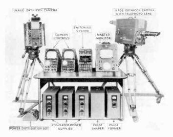
Figure 102. Field pickup camera chain. (courtesy RCA)
