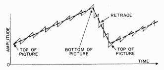
SOLID LINES - HORIZONTAL SWEEP SIGNALS DOTTED LINES - COMPENSATING SAWTOOTH
