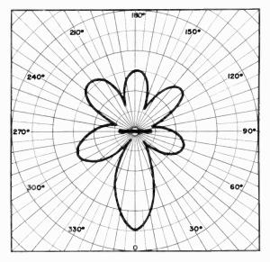
Figure 41. Field pattern of bat-wing antenna at 180 Mc.
