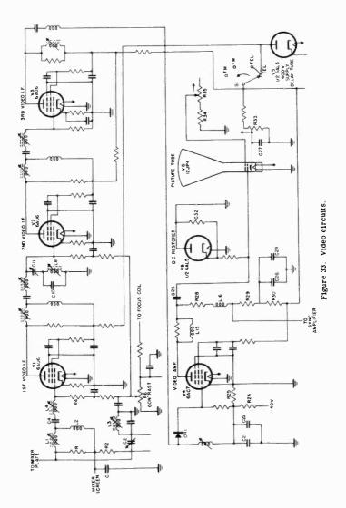
is developed across the positioning controls and focus coil which are in series with the ground return of the low voltage transformer. The divider consists of R24 and R25 and provides the proper bias for the video amplifier.
