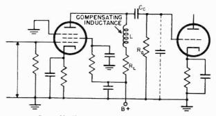
Figure 63. Shunt-peaking frequency compensation.
