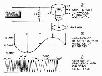
Figure 158. Simple method of frequency modulation.
