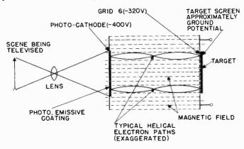
Figure 8. Multiplier section of the image orthicon.
