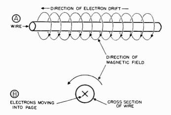
Figure 20. Direction of electron current flow in, and direction of magnetic field surrounding, a wire.
