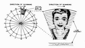
Figure 10. Rorating disc used in Nipkow's television system.
