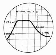
Figure 46. Video i-f response curve using tuned circuits only.
