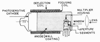
Figure 3. Construction of the image dissector.
