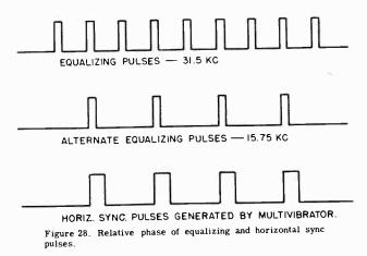
blanking pulses would not be distinguishable if the pulses were to occur close together.
