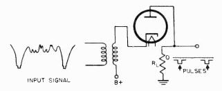
Figure 80. Diode sync clipper.
