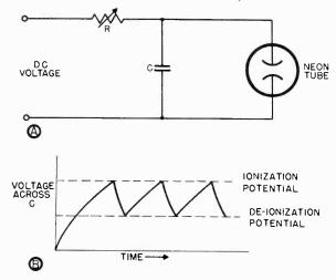
Figure 106. Simple electronic saw-tooth generator.
