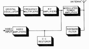
Figure 42. Block diagram of high level modulated transmitter.
