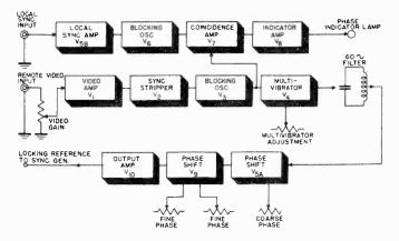
Figure 68. Block diagram of sync phasing unit.
