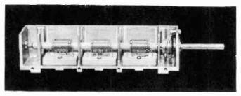
Figure 10. The Inductuner. (courtesy DuMont)
