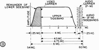
Figure 71B The bandwidth of a television channel is reduced to six megacycles by partially suppressing the lower side-band.
