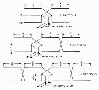
Figure 69. Center-fed flat-top arrays (top view).
