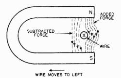
Figure 22. Wire placed at right angles to the lines of force from the horseshoe magnet.
