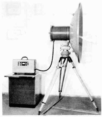
Figure 103. Microwave relay transmitter. (courtesy RCA)
