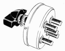
Figure 43. Coaxial switch. (Workshop Associates)
