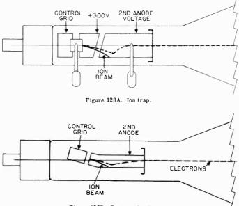
Figure 128B. Bent gun ion trap.
