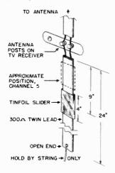
Figure 39. Simple wave trap.
