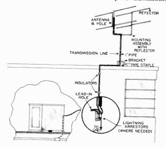
Figure 33. A typical installation.
