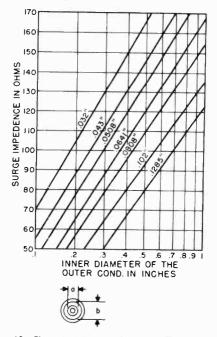
Figure 19. Characteristic impedance of coaxial transmission lines.
