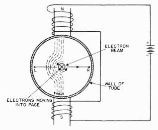
Figure 34. Method of magnetically deflecting the electron beam.
