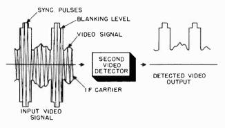
Figure 52. Input and output waveforms of the second detector.
