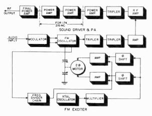
Figure 112. Block diagram of RCA sound transmitter.
