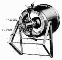
Figure 139. The optical barrel of the Philco projection system.
