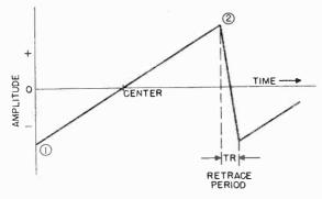
Figure 54. Sawtooth scanning voltage.
