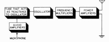
Figure 62. Block diagram of f-m sound transmitter.
