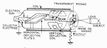
Figure 4. Construction of the orthiconoscope.
