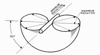
Figure 26. Radiation pattern of half-wave dipole in free space.
