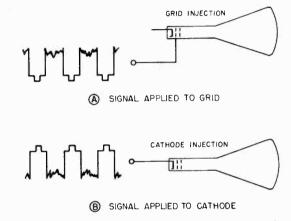
Figure 55. Polarity of signal required at grid and cathode of picture tube.
