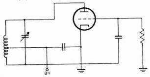
Figure 10. Series-fed Hartley oscillator.
