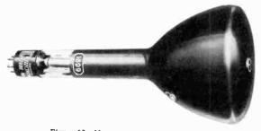
Figure 13. Monoscope tube. (courtesy RCA)
