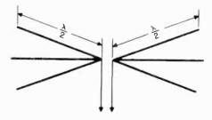
Figure 44. Full-wave fan antenna.
