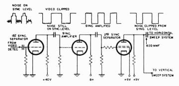
Figure 83. Cascade sync clipper.
