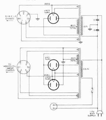
Figure 57. Low voltage power supply.
