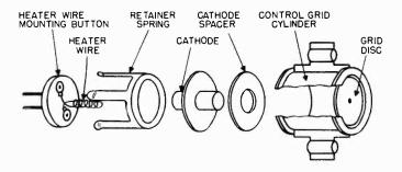
Figure 6. The cathode-grid assembly.
