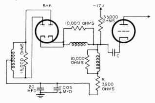
Figure 59. Push-pull video detector.
