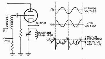
Figure 24. Stabilized blocking oscillator frequency divider.
