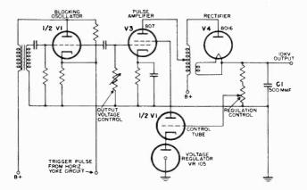
Figure 152. Regulated pulse type supply.
