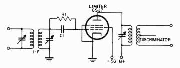
Figure 165. Simplified schematic of limiter circuit.
