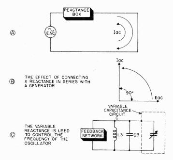
Figure 159. Operation of reactance modulator.
