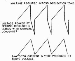
Figure 52. Voltage and current waveforms required for magnetic deflection.
