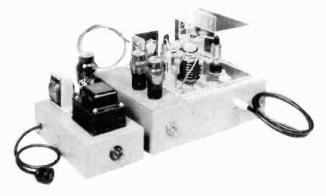
Figure 147. R-F high voltage power supply.
