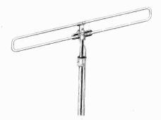
Figure 35. Folded dipole antenna. (courtesy Ward Products)
