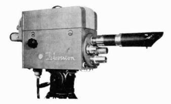
Figure 9. Studio camera equipped with lens turret.
