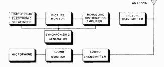
Figure 1. Block diagram of simple television transmitter.
