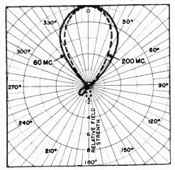
Figure 58. Field patterns of duo-folded dipole at 60 and 200 Mc.
