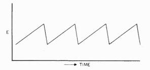
Figure 103. Waveform of current in deflection coils.
