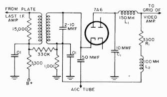
Figure 57. Schematic of video detector with bandpass filter.
