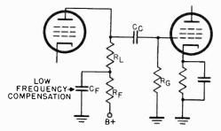
Figure 67. Parallel resistor-capacitor combination for low frequency compensation.
