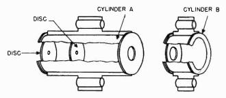
Figure 7. The pre-accelerator electrode assembly.
