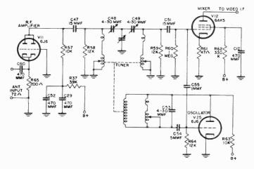
Figure 12. Schematic diagram of Inputuner.
