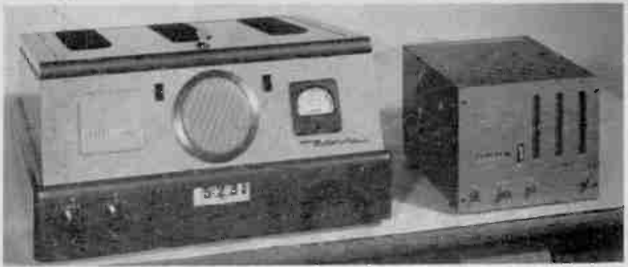
Complete recording station showing Motorola receiving equipment and scaler-divided unit for indicating count from remote radio-active snow gage stations.
