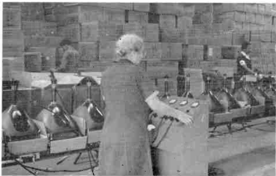
Life tests, above, are given on 17-inch zero-voltages electrostatic focus picture tubes at GE's plant at Electronics Park, Syracuse. Tubes, below, are being put through final electrical tests before shipment from the warehouse.
