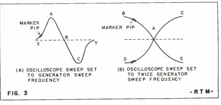
Scope traces found in FM alignment under ideal conditions. At (A), scope's sweep frequency equals generator sweep frequency. At (B), scope sweep is double that of the wobbulator.
