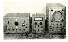
AM generator, sweeping generator, and oscilloscope, for the complete FM alignment procedure.
