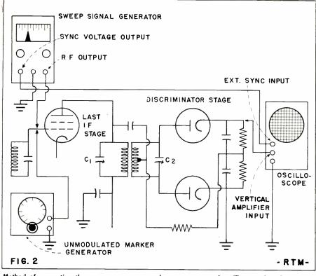
Method of connecting the sweep generator, marker generator, and oscilloscope for alignment of the FM second detector. See text for alignment procedure.
