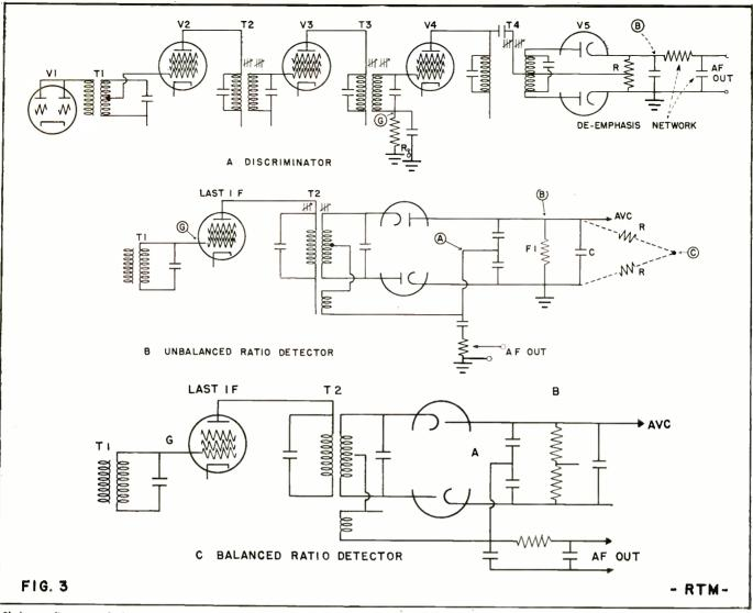
Skeleton diagram of the FM circuits, with some parts left out for clarity. The essentials are left in to show test points used in alignment of the set. The tests and procedures given in this method are more
