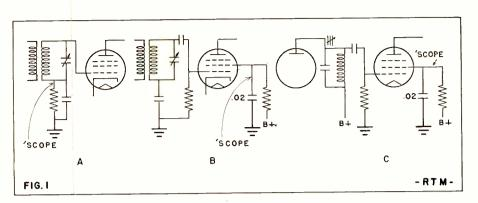
Different connections for FM limiter circuits. In (A), the normal 'scope connection has no effect on the limiter's input circuit tuning. In (B) and (C), however, the hot lead from the 'scope is coupled to the screen grid of the limiter tube by attaching it to a fine wire wrapped around the element's pin connection.
