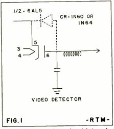
Crystal detector used for demodulation of a TV viedo signal. Use of crystals in place of vacuum diodes is increasing with TV design development.
