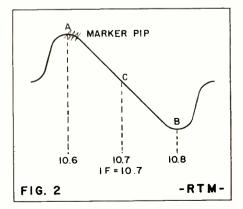
Optimum response curve at discriminator transformer secondary. Straight line between points A and B is desired.
