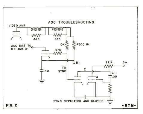
polarity of the signal. Sometimes the signal is DC coupled to the CRT and sometimes it is capacitively coupled. Whenever it is capacitively coupled there must be DC restoration; 3. The synchronization pulses are coupled to the grid of the sync separator tube and fed eventually to the horizontal and vertical oscillators.
