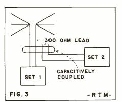
Emergency substitute for a two-set coupler. Leading lines from the two receivers are capacitively connected.
