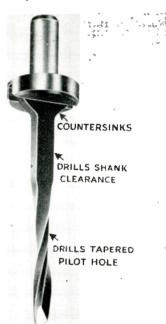
The shoulder on the tool stops the drill at just the right depth, while the size of the drill is slightly smaller than the body of the corresponding wood screw to provide a snug fit. Screw-Mates fit any drill gun, hand drill, or drill press and are available in a variety of sizes. For sizes, literature, and prices, address: D. R. Carner Co., Inc., 106 Hospital St., Providence, R. I.
