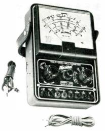
Battery operated, it provides 20,000 ohms per volt input resistance on DC, and 5,000 ohms per volt on AC. Voltage ranges AC and DC: 2.5, 10, 50, 250, 1,000 and 5,000.
