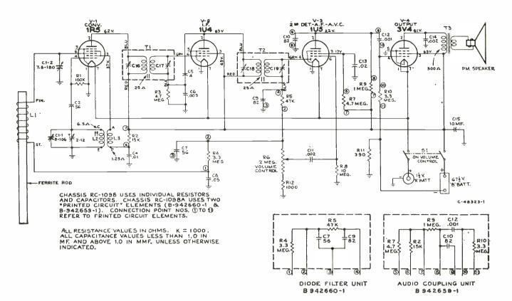
Schematic diagram of the new RCA "Personal" portable, a tiny fourtube receiver which is completely self-contained, yet is no larger than a popular novel, and weighs less than three pounds. Two printed cir-
