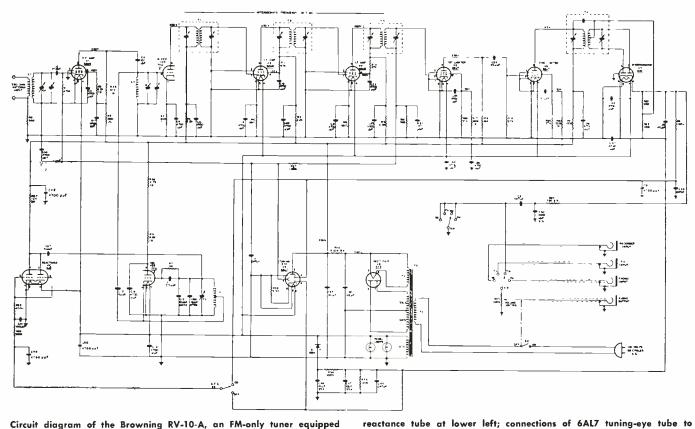
Circuit diagram of the Browning RV-10-A, an FM-only tuner equipped with tuning eye, automatic frequency control, and cascade limiters. Note duo-triode 6J6 with two triodes hooked in parallel as afc
