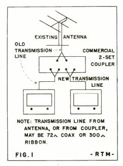
Circuit connections for two-set coupler, connecting FM and TV, or two TV sets, to a common antenna. Coupler is especially useful in apartment house installations or other multipledwelling installations.
