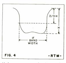
Ideal response curve to be obtained when aligning FM IF stages.
