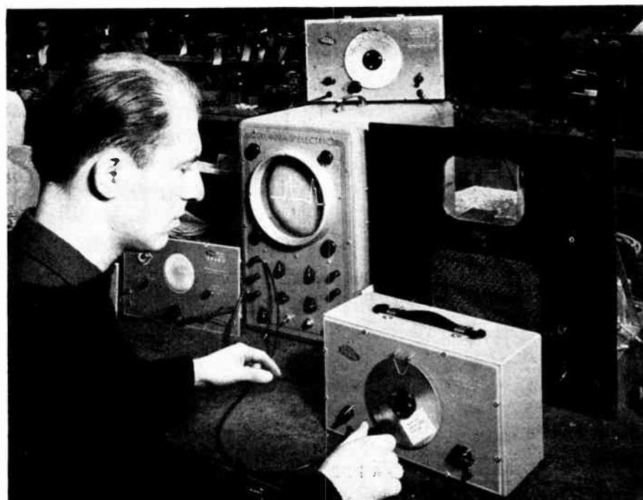
Fig. 1 This illustration shows one of the many factory tests—checking the pass-band of the Television Receiver (right) upon a scope (center) with the new Sweep Generator (front).
