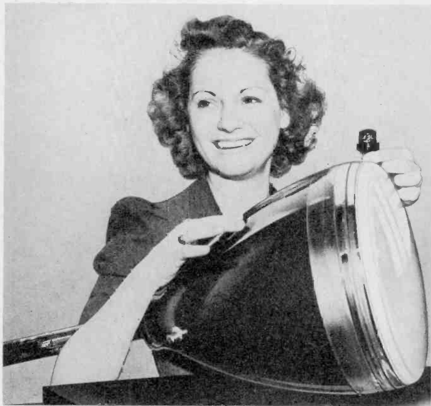
Fig. 3 An RCA cathode ray tube of the type used in television receivers. The girl is also holding a conventional metal tube to show the difference in size.
