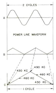
Fig. 1. Pyramid wave, B, developed from power-line sine wave, A; and output frequency variation, C, over one cycle of line voltage. from this, the audio modulation from a broadcast transmitter is rarely constant over any length of time. For these reasons, a calibrated signal source with controllable output, and some method of accurately measuring the output of the receiver is required. This latter may take the form of an A-C meter across the voice coil of the speaker; or a vacuum-tube voltmeter
