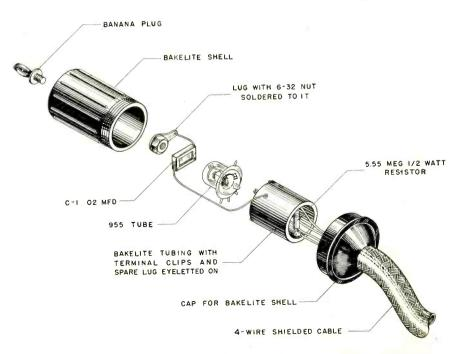
Fig. 4. Exploded view of probe showing construction for use with 955 tube.
