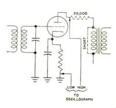
Fig. 6. Connections of oscillograph to biased detector, showing addition of resistor in plate circuit, and short across coupling transformer.
