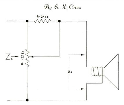
Fig. 1 Method of connecting simple wire-wound potentiometer and additional resistor to make a pad which approaches constant-impedance characteristic.
