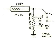
Fig. 1. Simplified input circuit of RCA Volt-Ohmyst.
