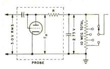
Fig. 3. Simplified input circuit for modified RCA Volt-Ohmyst.
