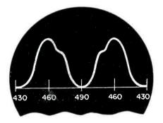
Fig. 2. Appearance of output of improperly adjusted I-F amplifier with oscillograph sweep synchronized at the power-line frequency.
