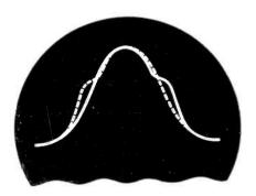
Fig. 3. Same I-F response as in Fig. 2, but with oscillograph sweep synchronized to twice the power-line frequency. The solid line indicates the response for the upswept half-cycle; the dotted line for the down-swept half-cycle.
