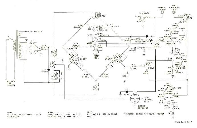
Fig. 5. Complete circuit of RCA Volt-Ohmyst as modified for use as high-frequency A-C voltmeter.
