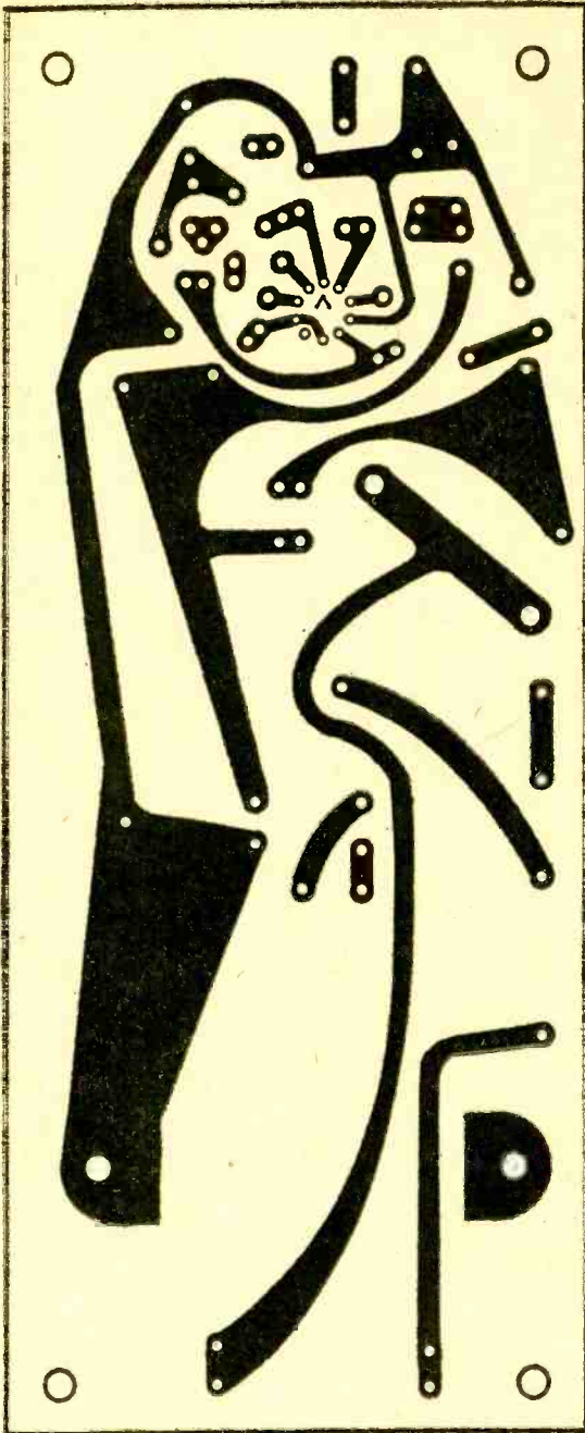
Circuit board for Lover's Lamp appears here exact size— 6\frac{3}{4} \times 3\frac{3}{4} in. Small V within 10-pin circular configuration at busier end of board indicates pin 1 of integrated circuit IC1. See text for information re sizes of bits to use for holes.
