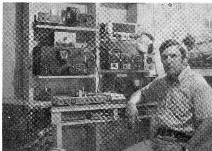
Al Cikas, Springfield, IL is into an off-beat form of DXing, monitoring the video pictures of amateur radio slow-scan TV (SSTV). (See text.) Al has constructed an adaptor (flat unit on desktop) to convert an oscilloscope (left foreground) to receive the video signals.
