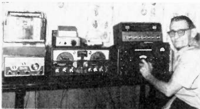
Now here's a well equipped DX shack, belonging to retired Navyman Joseph Helm, Odon IN. The receivers shown, from left, are a South African portable, the Barlow Wadley XCR-30, atop a Drake SPR-4; Hallicrafters SX-100, with the Gilfer Associates A-20 preselector on top; Realistic DX-150, on top of the "big boy," a Collins R-388/URR.
