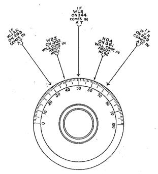
Suppose you want to get WBZ. Suppose WJAX on 263 meters comes in at 30. Suppose WLS on 344 meters comes in at 50. Then WBZ on 302 meters, or half-way be-
