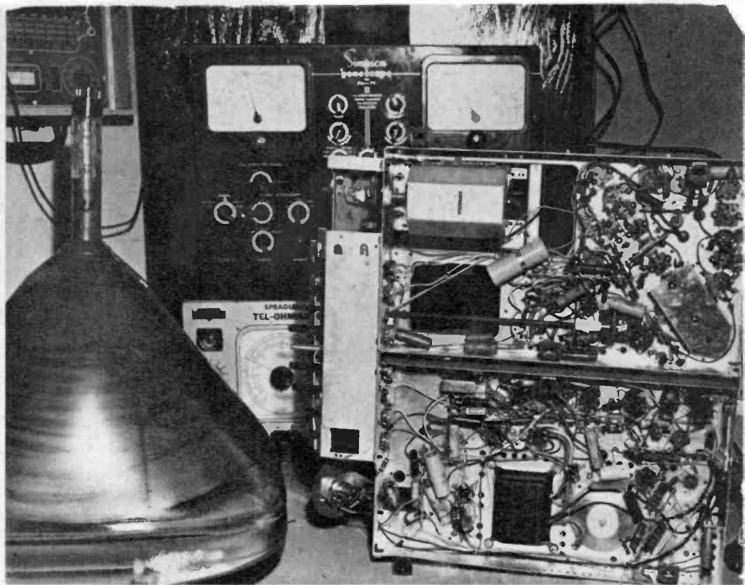
THIS CANDID SHOT shows a picture tube, upright (left front); a panel housing TV test equipment (background); a bottom view of a television chassis showing a part of the multitude of components in your receiver.
