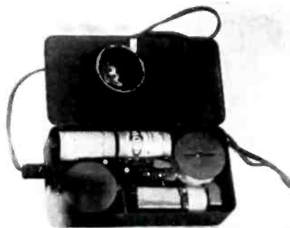
• An interior view of a pocket-size magnetic recorder built by Armour Research Foundation scientists. It is the only one of its kind.
