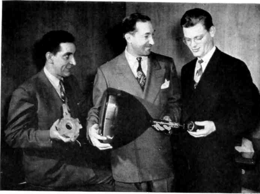
Asher J. Cole, left, president, National Video Corp., beams his approval of his firm's new tube, which is designed to save four and one-half thousand tons of copper a year. Holding the tube are co-inventors Edgar W. Morse and C. V. Fogelberg, center and right. The new tube permits focusing without the use of a focus coil.
