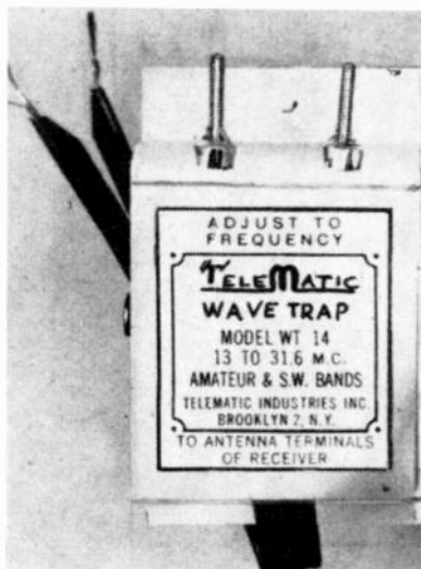
This wave trap is from the Telematic detection kit.
