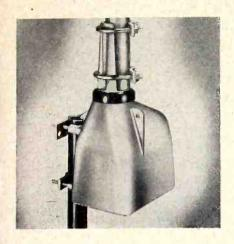
This new antenna rotator drive motor features 5/8-inch steel drive shafts, 3-inch final shaft steel gears for added strength and turning power. Available with mahogany-finish control box with "Electric Eye" to flash position, or "Compass" which gives reading of antenna position.
