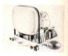
Featured in this television kit are quickaction keyed AGC circuit, "hi-sweep" voltage multiplier system, 12-channel turret tuner, full 4 mc. band width. Kit comes in one model with principle components mounted, in another unassembled. Comes with components, picture tube mounting brackets, speaker and tubes (less kine, wire and solder).
