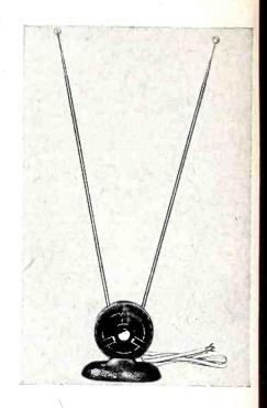
The three-section, triple-chrome plated telescopic dipoles on the "Tip-Proof" antenna can be adjusted from 15 to 41 inches for rapid orientation. Tension design holds dipoles at any position. Base is balanced and weighted to prevent antenna from tipping or rocking. Made of engraved satin finish mahogany plastic.
