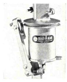
Of aluminum construction and with weather-sealed ball bearing working parts, this TV antenna rotator is operated through a worm-gear control box attached to the outside of the hcuse. Turns antenna 360 degrees. Positions lock automatically, and metering device provides easy and speedy selection of chosen stations.
