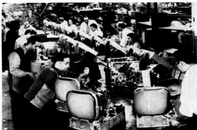
An assembly line at the Air King Products Co., Inc. modern plant in Brooklyn, N. Y. With over 200,000 square feet of manufacturing space, Air King manufactures radios, wire recorders and television receivers. TV production is expected to reach new highs in 1950, and the firm recently announced full capacity production of its 16-inch rectangular tube TV models.
