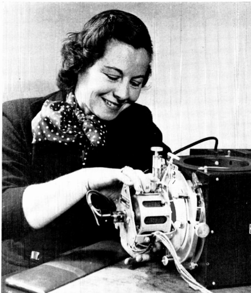
Focusing the Protelgram projection unit is not at all complex. Here Virginia Forsythe, on the public relations staff of North American Philips, rotates the complete "tail piece" slightly. Even inexpert, feminine hands can make this corrective adjustment if the picture slants or leans to one side.
