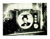
The 12½-inch picture tube in this table model television receiver provides an 89-square-inch screen. Automatic frequency lock keeps image steady, and gain control eliminates station-to-station adjustments. Set has 8-inch speaker and is equipped with phono jack for any type record changer. Cabinet is mahogany veneer.
