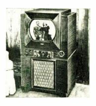
A television receiver with a 16-inch direct-view tube, which furnishes a viewing screen 145 square inches in size. Chassis contains 31 tubes. Full coverage on 12 channels. FM sound system, two stages of video amplification and noise saturation circuit. Uses 10-inch Alnico V PM speaker. Console cabinet is in maliogany veneer.
