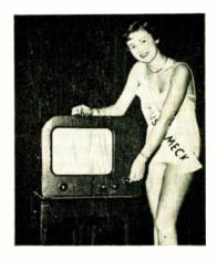
This television receiver provides 65 square inches of picture with a 10-inch cathode-ray tube. Has 17 tubes and two rectifiers. The tubes used are dual and triple section ones, performing the functions previously done by two or three separate tubes. Cabinet is hand-rubbed mahogany, with rounded sides.
