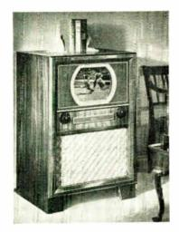
This mahogany console utilizes a 121/2inch cathode-ray tube and is one of four television receivers introduced as the latest Arvin line. Sets include two consoles and two table models. Table models have 10- and 121/2-inch tubes, and the second consale uses a 16-inch tube. Matching tables for the table models are available at extra
