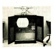
To give its 203 square inches of picture space, this television console uses the new short-necked 19-inch cathode-ray tube. Instrument contains full-range FM radio and plugin receptacle for record player. Has firm's local-distant switch and two-speed square selector dial. Set has 25 tubes and five rectifiers. Cabinet is made of maliogany veneers.
