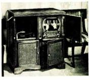
Screen on this television console combination is 63 square inches. Set uses a 10-inch picture tube, and features all-channel reception, built-in antenna and new discriminator circuit. AM-FM radio has 10-inch speaker. Record player handles all speeds and all sizes of records automatically.
