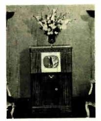
Model 661P, a new Capehart console television receiver, has a mirrorbacked, flat-faced picture tube which assures high-definition 54-squareinch images that can be viewed in full daylight. Has 12-inch high fidelity, permanent magnet speaker, and includes 24 tubes and four rectifier tubes in addition to the viewing tube. Mahogany cabinet is of 18th century English design and is suited as a companion piece to a Capehart phonograph-radio. Stands 42 inches high, is 19 inches wide and 21½ inches deep.
