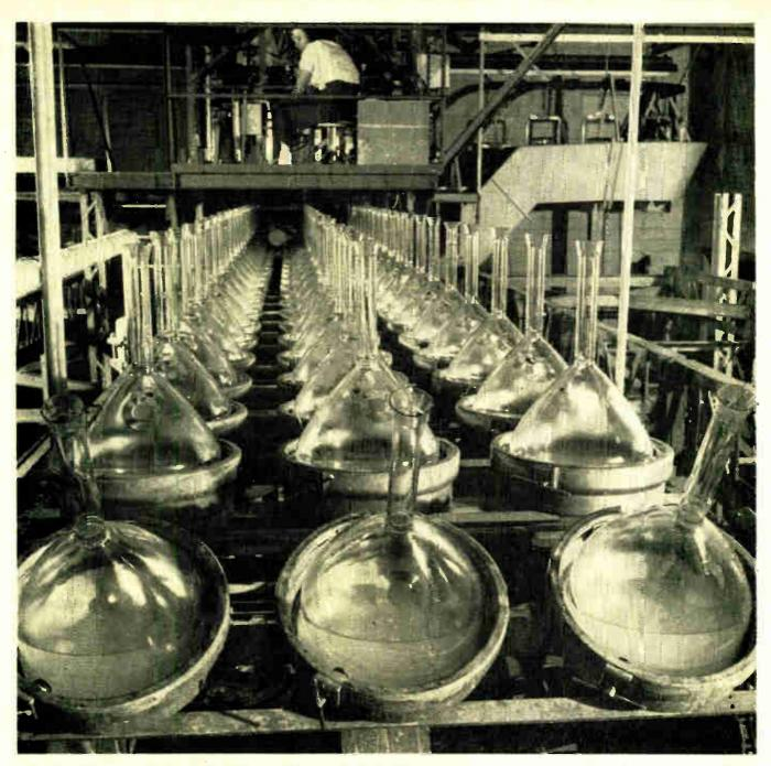
Symbol of industry of future, glass bulbs marching on conveyor lines, to emerge as kinescope picture tubes for TV receivers. Production rises or falls with every fluctuation of these mass-produced tubes.
