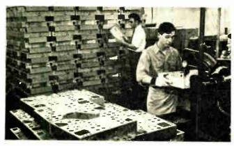
Joining sockets, terminal boards, and condenser wafers to chassis on rivet press. Inspector in rear examines each.
