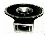
To meet the demand for a reproducer to convert existing equipment for high fidelity, this newly-designed Tru-sonic Model P-52FR speaker has a frequency range from 40 to 14.000 cycles. Supplied in both 12" and 15" cone diameters and equipped with 2½ pounds of Alnico V magnet material.
