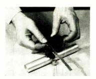
A unique new lightning arrestor. designed to fit quickly and easily into television and FM receiver installations. This simple plastic and metal device will fit 300-ohm transmission lines and is a foolproof new method of attaching the transmission line which avoids cutting and splicing. The arrestor is easily mounted on any indoor water pipe by means of its flexible metal ground strap.
