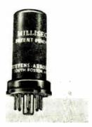
This Milleseo Relay has an operating time as short as 1/3 milliseconds; it is assembled in a metal radio tube container with an 8-prong octal base, but its operation is mechanical rather than electronic. Previously, these relays were made in one size only, but due to the demand for multiple pole eonstruction, this firm is now offering these relays in the same container except double pole, double throw.
