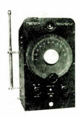
A Frequency Meter especially designed for measurements in the 72-76 and 152-162 megacycle band, this new meter features accuracy in either band of .005%, or .0025% where minor precautions are taken. A whip antenna mounted at the side of the cabinet furnishes coupling to the transmitter and may be telescoped to form a convenient carrying handle. Operates from 117 volts, AC or DC.
