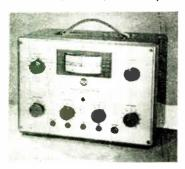
A new portable sweep generator designed exclusively for servicing and alignment of FM equipment. Type WR-53A furnishes all the signals needed for the complete alignment of frequency modulated radio receivers. Provides a signal tunable over the 88 to 110mc band, unmodulated or amplitude modulated, for the alignment of r-f, mixer, and local oscillator circuits.
