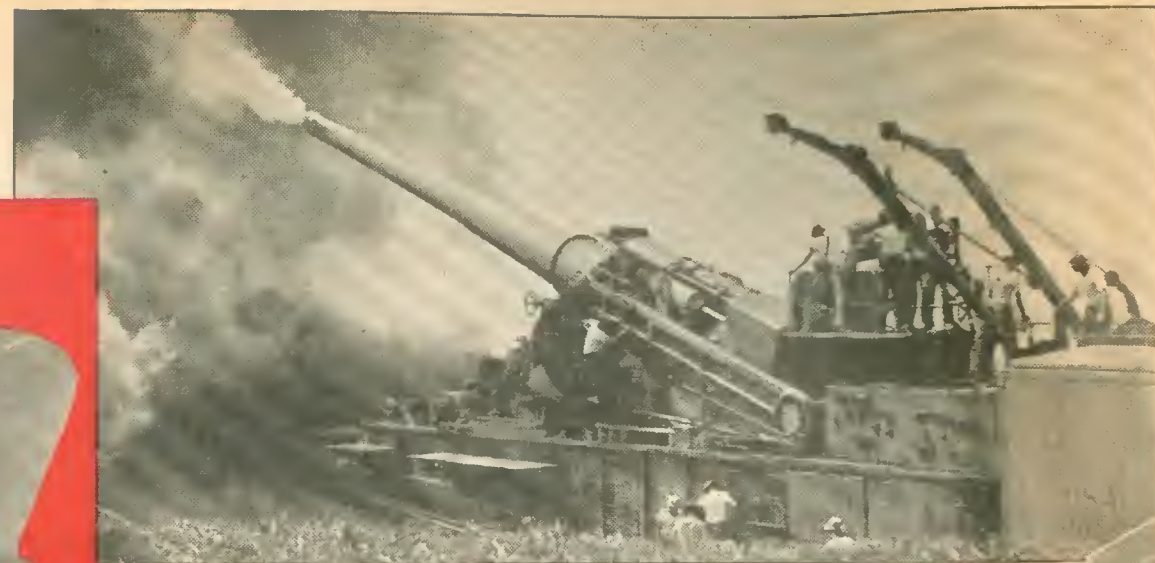
BIG BERTHAS of 1940, these fourteen-inch railway sea coast defense rifles will defend Panama Canal and U. S. coastline if America enters the war
