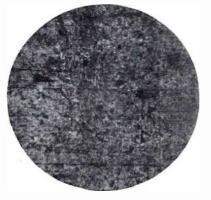
Flat strip of nickel for radio: Surface with no polishing or etching (100X unretouched). Note relative porosity and non-uniformity of surface.
