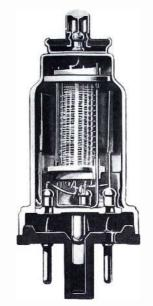
(Courtesy Raytheon Production Corp.) Interior structure of representative metal tube, cut away to show the positions of the elements.
