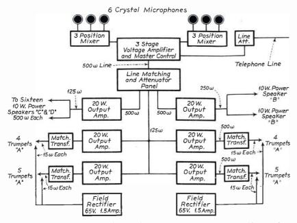
Block diagram of the amplifiers showing the grouping of light-weight portable amplifiers to develop the volume of power needed. It was necessary to use the four types of speakers and baffles to properly cover the area designated.
