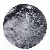
Nickel, after 150-hour bath in mercury at room temperature (60X).
