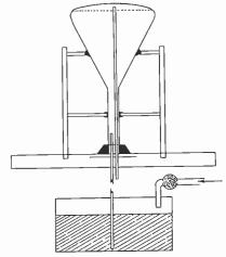
Fig. 2. A trap containing sodium hydroxide in the pressure-line to the reservoir absorbs gaseous acid-anhydrides, thus preventing the formation of electrolytes in the graphite solution.
