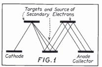
Illustrating the functioning of the electron multiplier tube.
