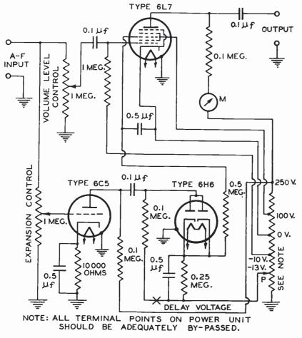
Fig. 1. Volume-expander circuit using a 6L7 tube.
