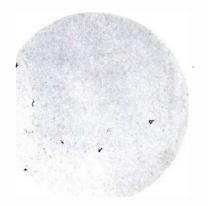
Flat strip of Svea metal for radio: Surface with no polishing or etching (100X unretouched). Note uniformity with freedom from slag, impurities and gas bubbles.
