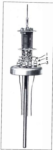
(Contress Raytheon Production Corp.) Structure of the 6Q7. The mica spacer (1) which supports the diodes, is sprayed with liquid ceramic for the purpose of improving insulation. The beads (2) are also sprayed with a liquid ceramic. Small rings of copper (3) are brazed onto the Fernico eyelets to prevent leakage.
