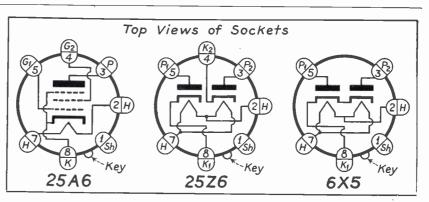
The third new metal tube is the type 6X5, a narrow space, high-vacuum rectifier designed primarily for automobile receiver use.
