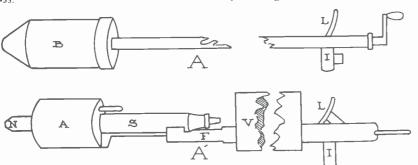
Fig. 3. (A') By pulling the lever L the intake I and the nozzle N open, as the section S moves back and forth on F. The chamber A contains the binder material, while V is a vacuum space. (A) By opening the valve by means of L and rotating the crank slowly, the fluorescent powders in B are forced out by the pressure of  $\frac{1}{2}$  to  $\frac{3}{4}$  atmospheres. Overall length of guns, 12 inches. (*Courtesy of Pfalte & Baucr.*)
