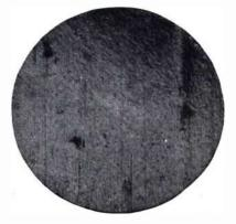
Special strip of purest domestic iron for radio: Surface with no polishing or etching (100X unretouched). Note impurities and elongated gas bubble under surface at right. Slag and carbon hard spots make uniformity impossible.
