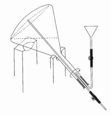
Fig. I. Funnel method, as employed in this country on both an experimental and small-production scale, for coating the interior walls of cathode-ray tubes.
