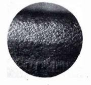
Lower Center: Specially prepared best quality domestic iron showing chemical action on the streaks of impurities—usually pockets of gas under the surface of the metal.
