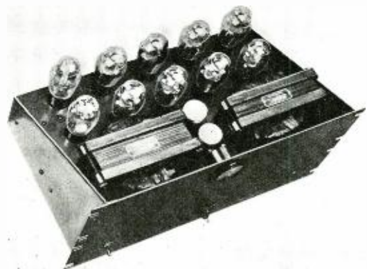
Fig. 5. The Lafayette 100-watt audio amplifier and power unit for rack mounting.
